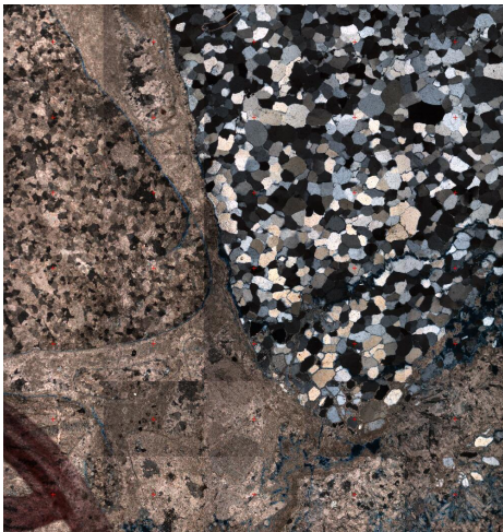
Figure 2.4. Pictures of conglomerate member of the fluvial system in thin section and outcrop. This sample was collected 80 feet up the section from the base. It is mainly composed of Ely Springs and Hidden Valley Dolomite and Eureka Quartzite.
