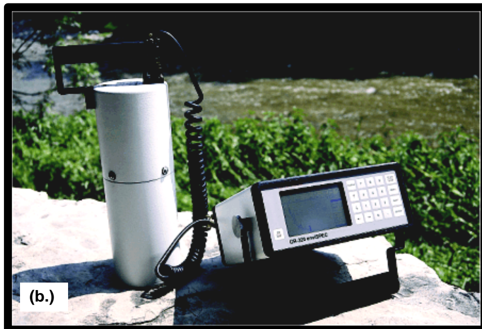
Figure 12. Study instruments. These portable instruments, used in the study were (a.) the MS2K manufactured by Bartington Industries, used to measure magnetic susceptibility (MS) and (b.) the Exploranium 320, used to measure gamma-ray magnitude and individual concentrations of gamma-ray specific elements. Both instruments allow rapid and non-destructive measurements of outcrop lithology in situ .
