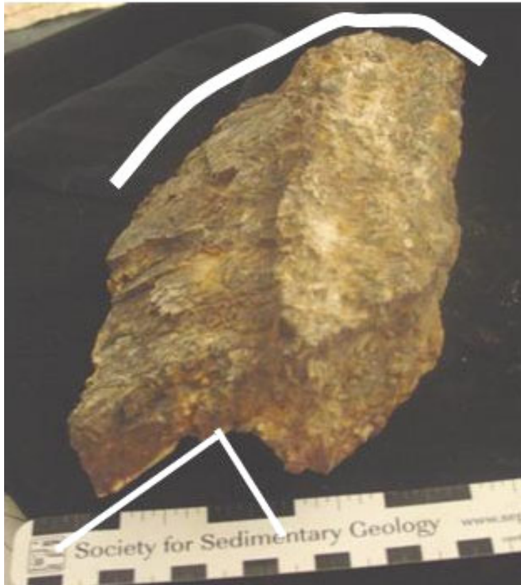
Figure 24. Pulverized, warped and welded siliceous welded breccia from ( Ph R ) partial repeated section north of spillway at Hass B. This pulverized welded siliceous shale (a.) is highly indurated and deformed. Original bedding planes of siliceous beds in (b.) are bent nearly 90°
