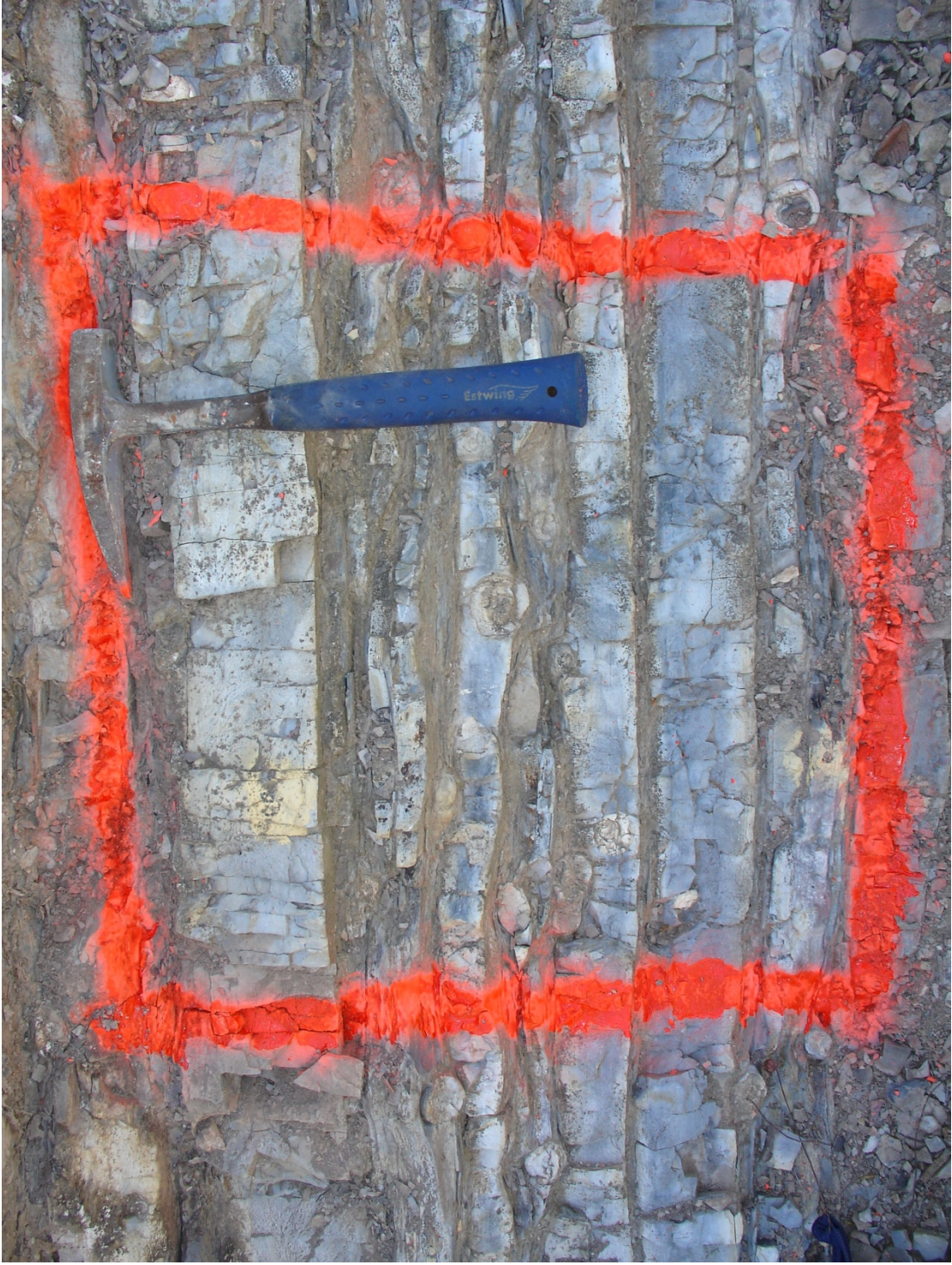
Figure 55. The upper level inventory square for the Woodford Shale I-35 South outcrop. The Phosphatic horizon with phosphate nodules and the cherty-silica rich beds are densely fractured. Notice that non-fissile units contains abundant amounts of perpendicular fractures.
