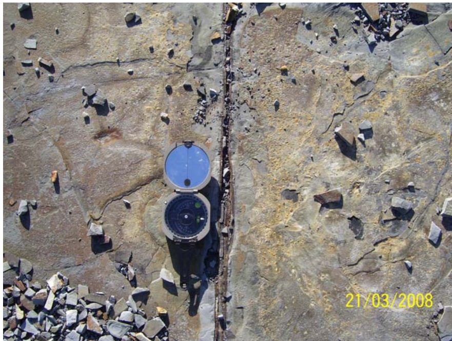
Figure 101. The fracture aperture of the Set I fracture. Clarita Shale pit 4-5 mm fracture aperture when the fracture spacing is around 70 cm.
