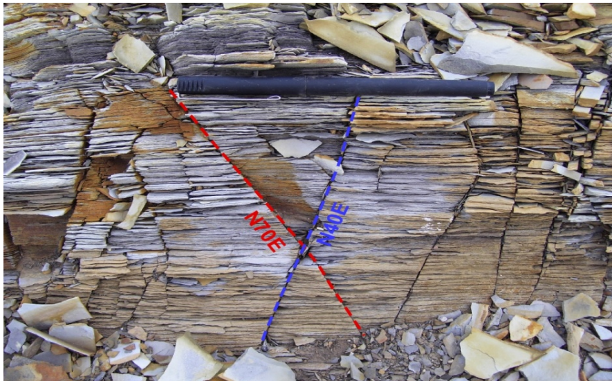
Figure 72. Dominant fracture sets striking N70E and N40E intersect at an acute angle within the bedding along the Woodford Shale at McAlister Shale pit outcrop.
