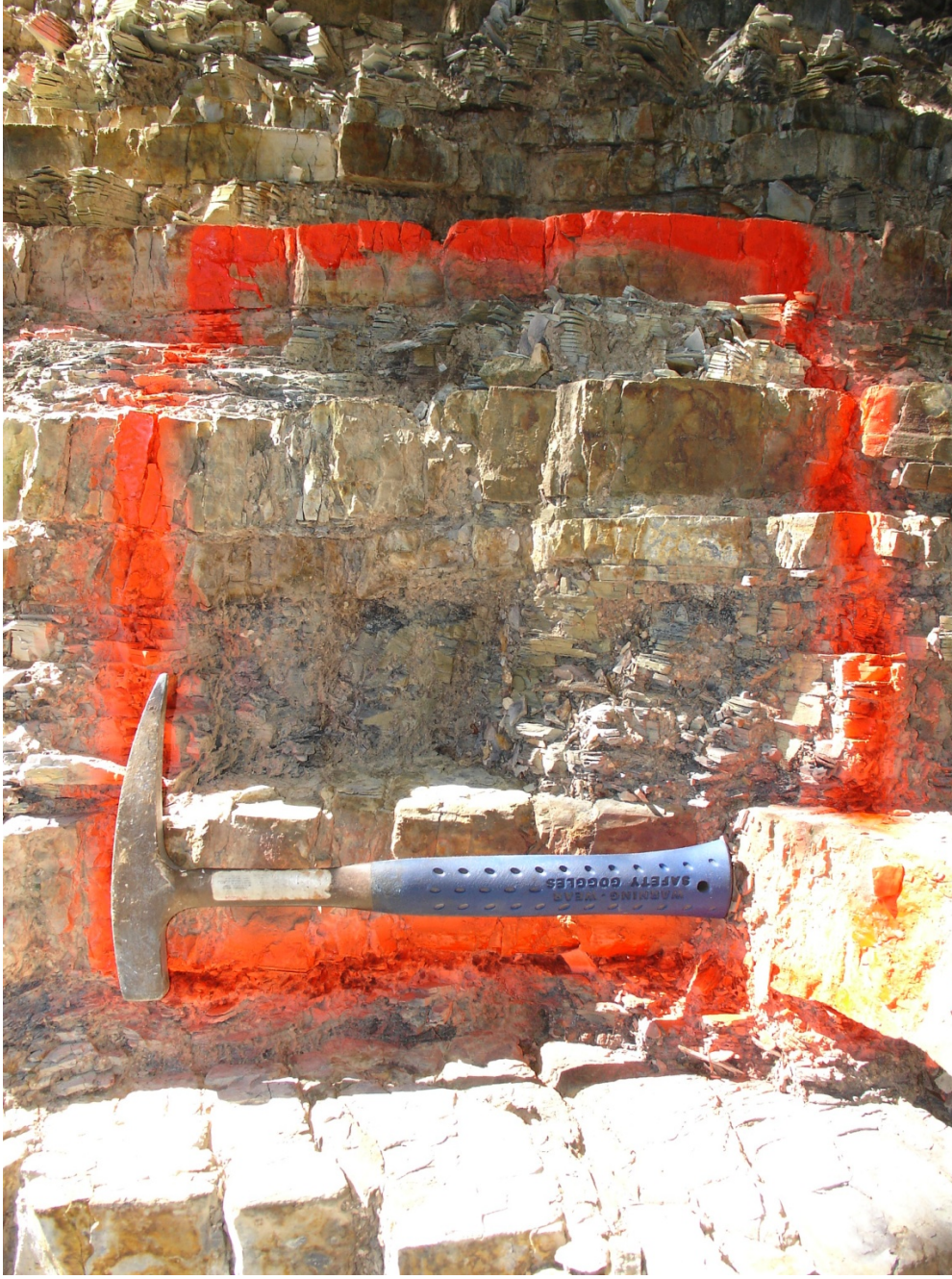
Figure 46.77D/ I35 North Outcrop: Inventory Square 1. that is perpendicular to bedding planes. This inventory square contains the organic-rich and the silica rich beds. Thin sections of the dark colored beds could not be prepared because of bed fissility and weakness.
