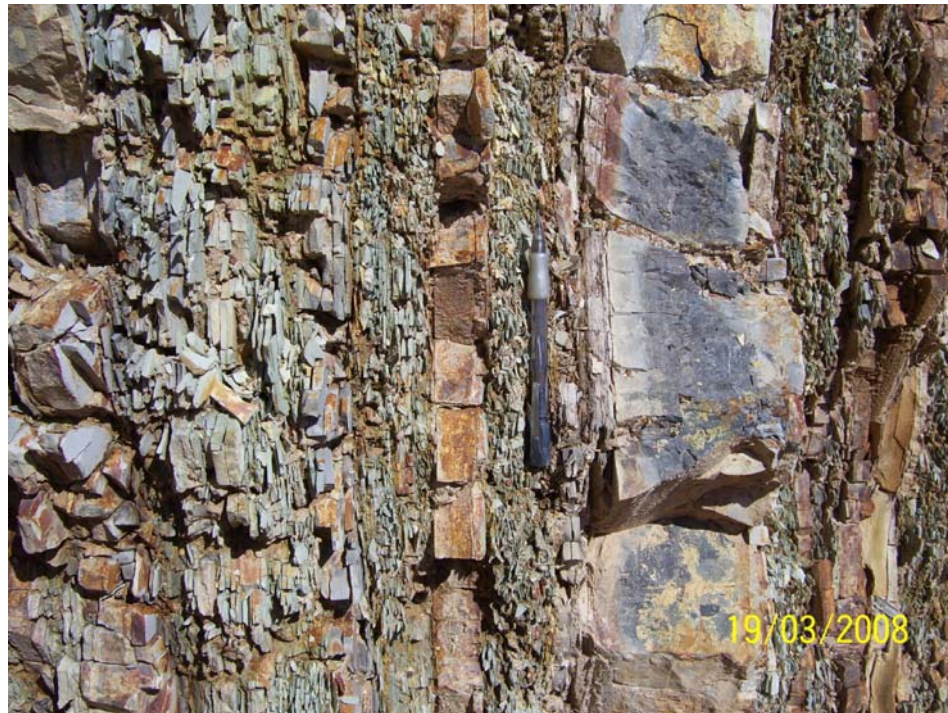
Figure 87. Fracture distribution for different mechanical units. Bed thickness is the major factor controlling the fracture distribution and development.
