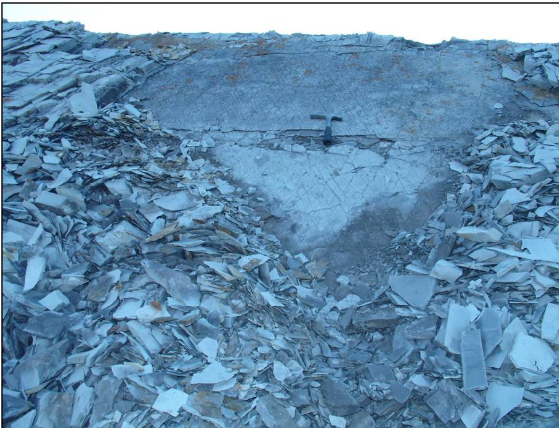
Figure 68. A section from the middle of Mc Alister Cemetery outcrop. The interval is silica rich and contains fissile and the non-fissile units. These units are fractured; and contain dead oil within the fracture sets.
