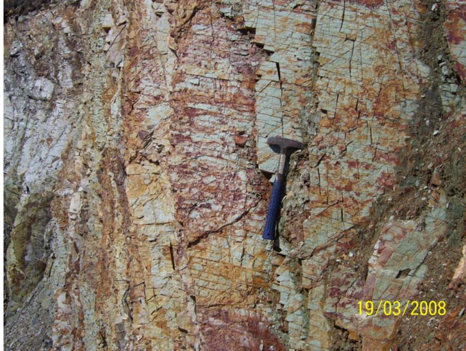
Figure 80. Close up view of well developed fracture sets. Notice that their dip change along the length of the fracture.
