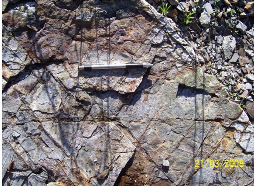
Figure 92. Fractures sets forming a conjugate pattern. In this cases the strike perpendicular fractures have not developed. The absence of strike perpendicular fracture may be because of the shear movement along the fracture sets.
