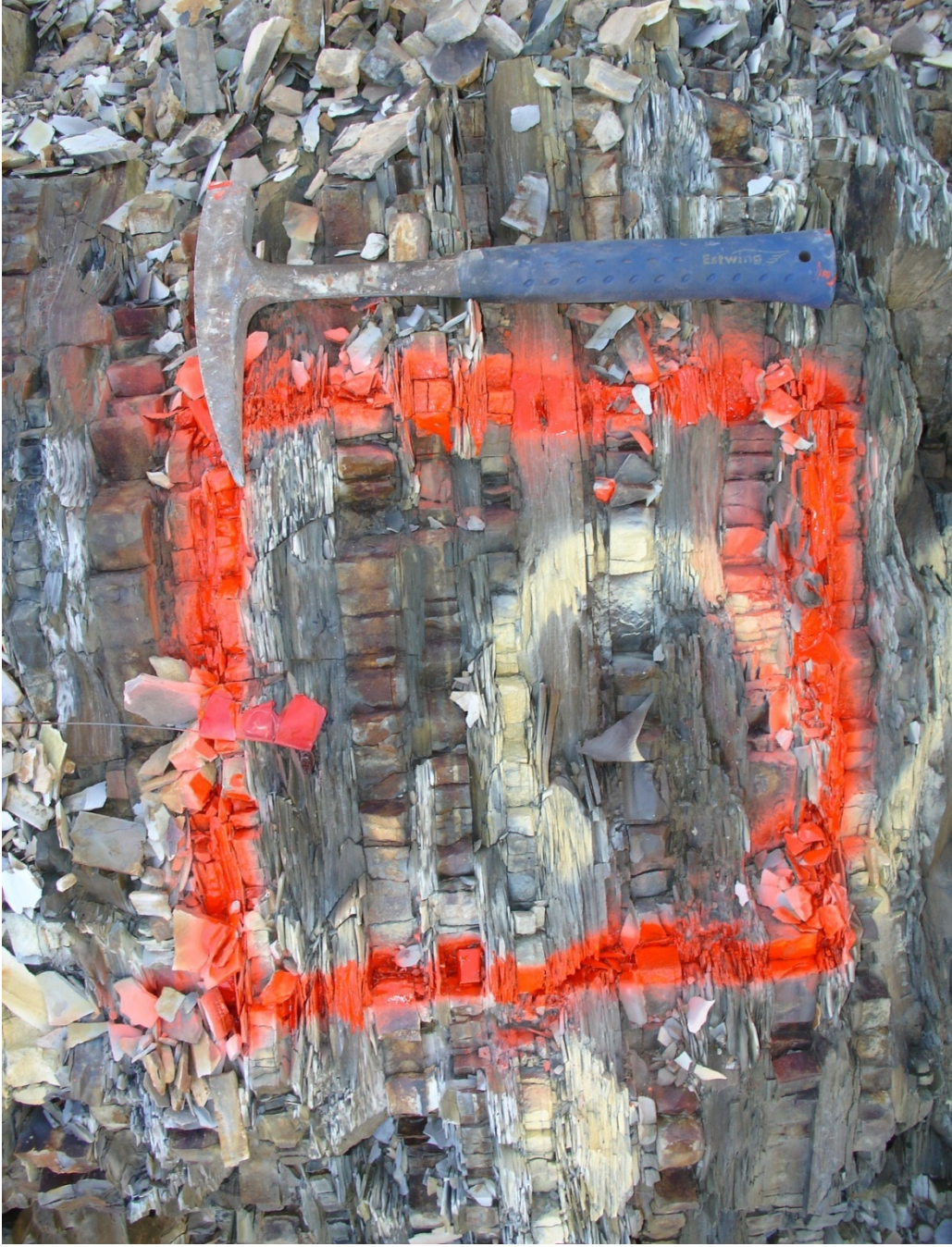
Figure 59. The lower level inventory square I-35 South Outcrop. The Fissile units and non-fissile units are darker colored than that of the upper inventory square. Non-fissile units are more silica-rich than fissile ones. Also notice that fissile unit fracture are rare and align oblique to bedding whereas non-fissile unit fractures are more common and perpendicular to bedding.
