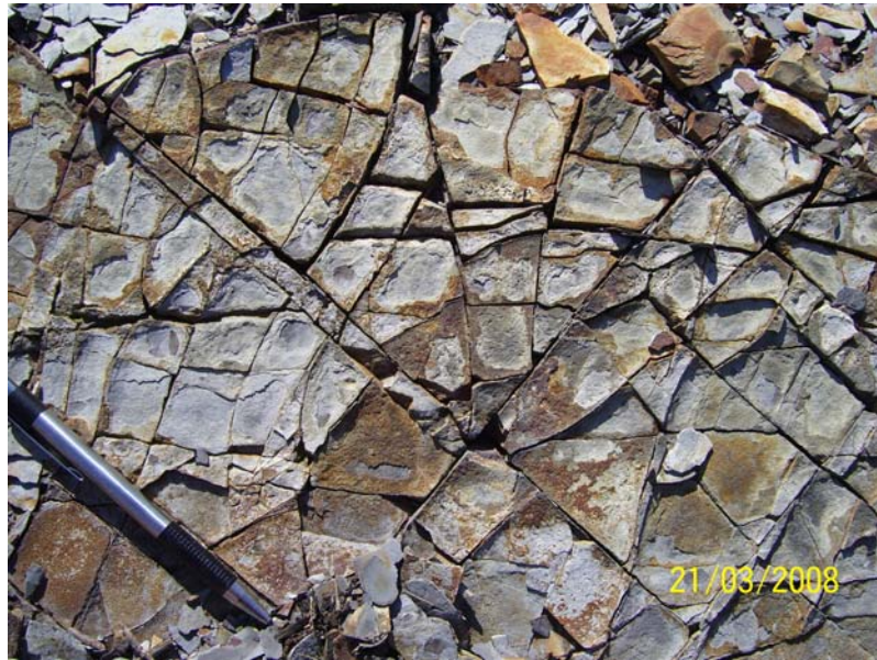
Figure 91. Fracture patterns for the Woodford Shale, Wapanucka Shale pit. Set II strikes N15E and Set I strikes E-W to form an orthogonal pattern. Notice the curve of strike perpendicular fractures and strike parallel fractures.
