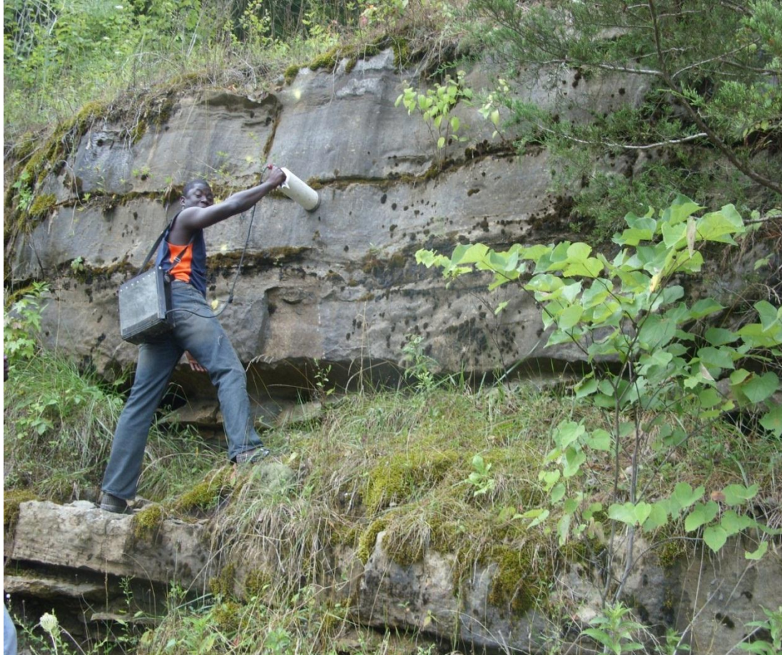
Figure 22: Photograph of Peyton Creek outcrop, Arkansas showing massive carbonate upper part of Pitkin Limestone. Note the irregular bed contacts and the gamma spectrometer
