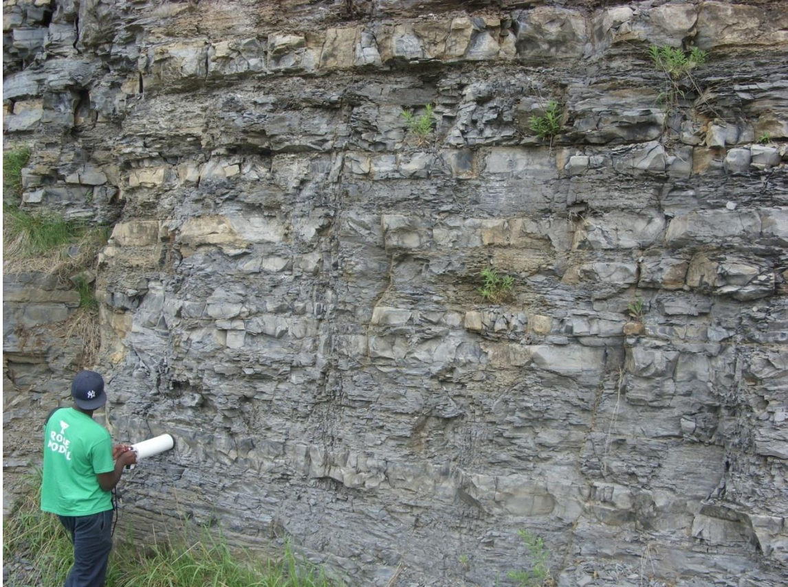
Figure 8: Marshall Outcrop showing the gamma ray spectrometer in use. Note the rugged handy detector mounted against the surface of the rock to measure any emitted radiation by the rock
