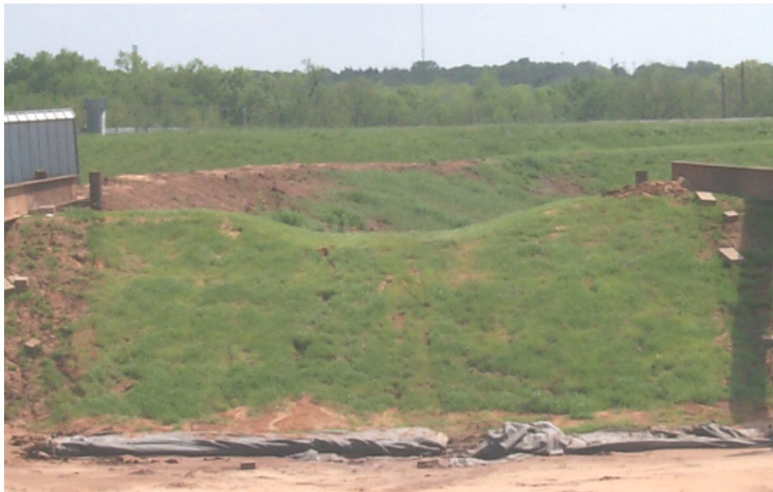
Figure B.1. ARS Test 1 embankment before overtopping experiment.
