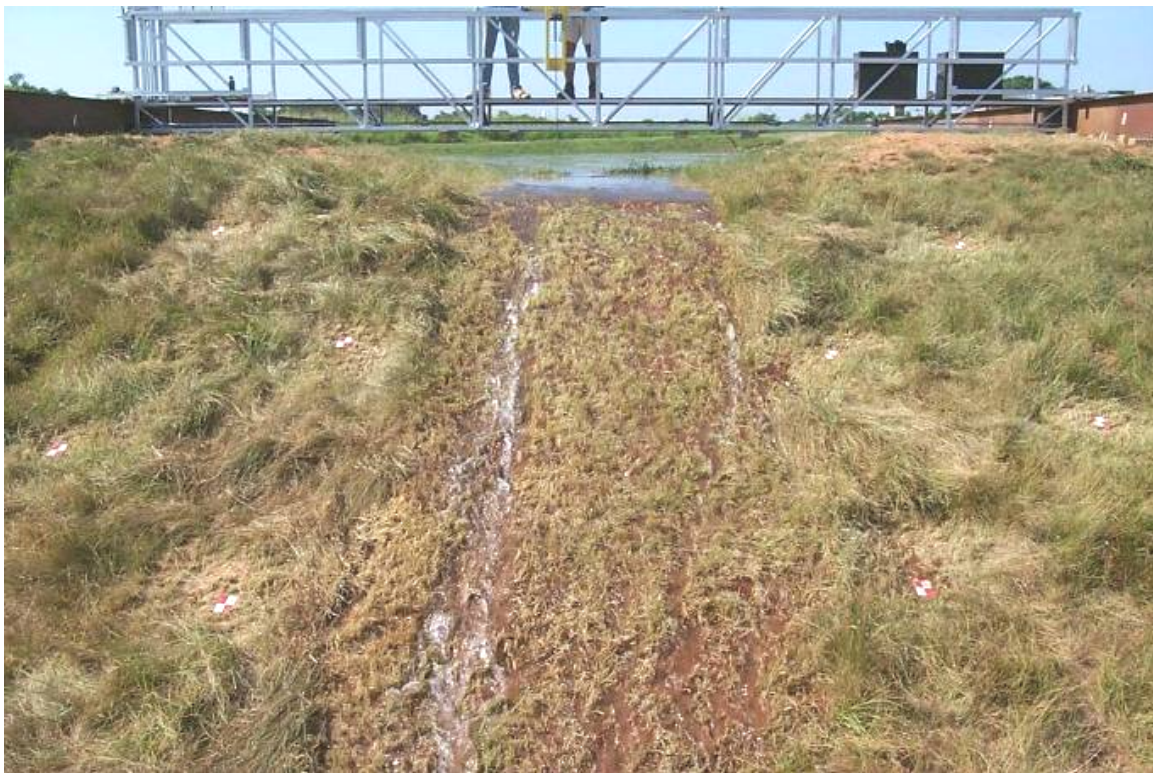
Figure C.1. ARS test 2 in first minutes of flow over crest.
