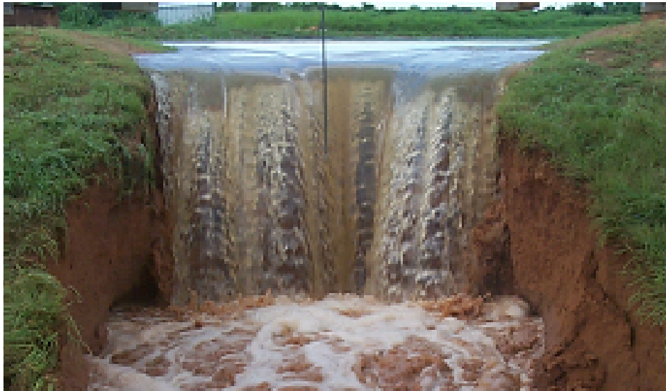
Figure 1.6 Downstream view of embankment overtopping experiment conducted by USDA Agricultural Research Service, Stillwater, Oklahoma in 1998. The observed steep overfall and migrating headcut are typical for embankments of cohesive material.
