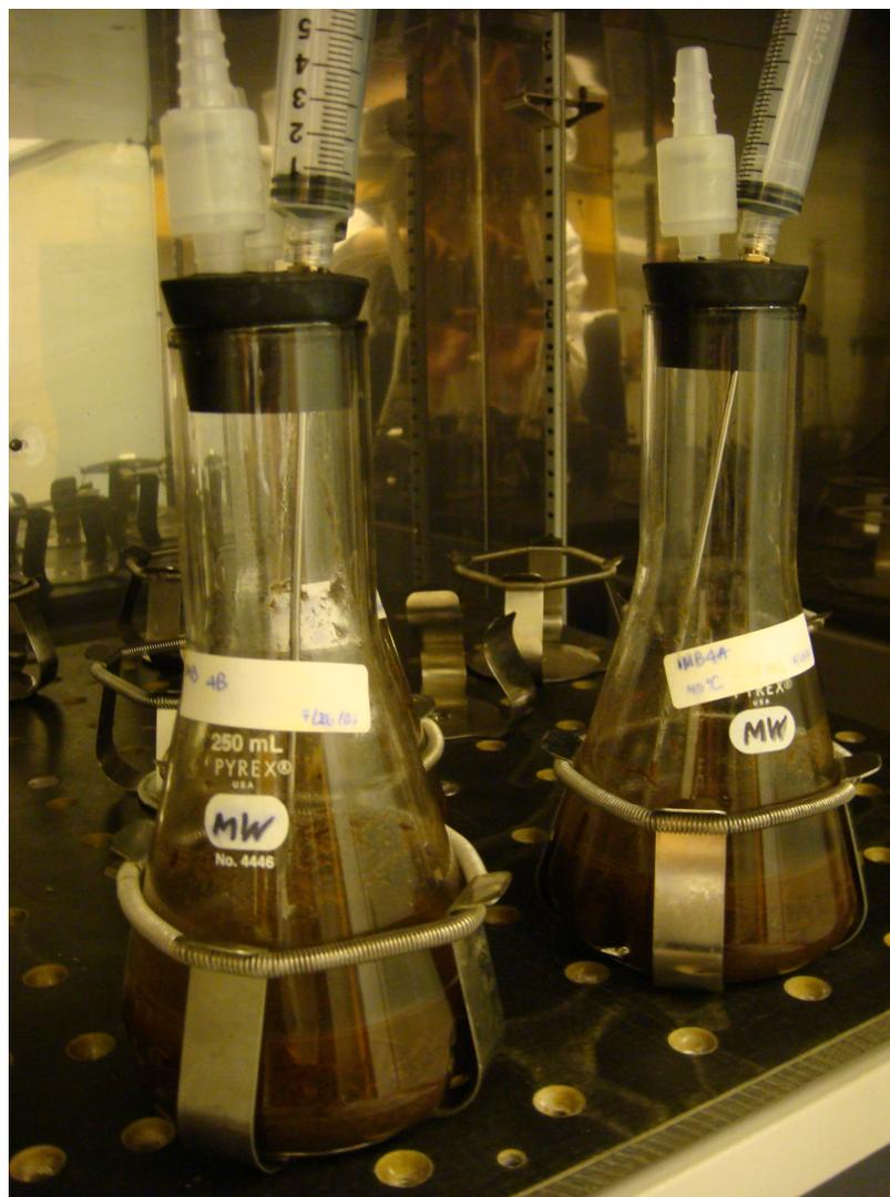
**Figure 4.2 Experimental set up of SSF of hydrothermolysis-pretreated switchgrass at 45°C using orbital shaker agitated at 130 rev/min.**
