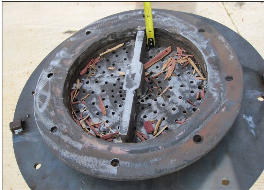
Figure 13: Bottom section of gasifier unbolted and removed showing grate and scraper
