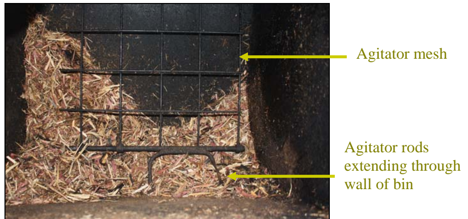
Figure 11: Internal view of hopper bin showing agitator.
