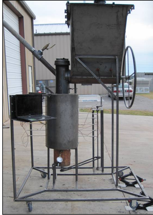
Figure 19: Gasifier showing support frame fabricated of one-inch (2.5 cm) square tubing.
