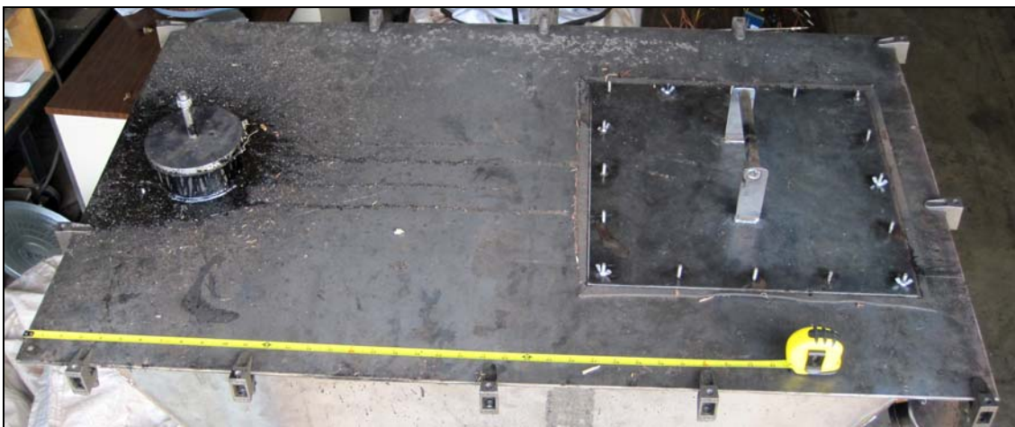
Figure 9: Top view of hopper showing secondary door, pressure release valve and C-clamps sealing top to bin during operation.
