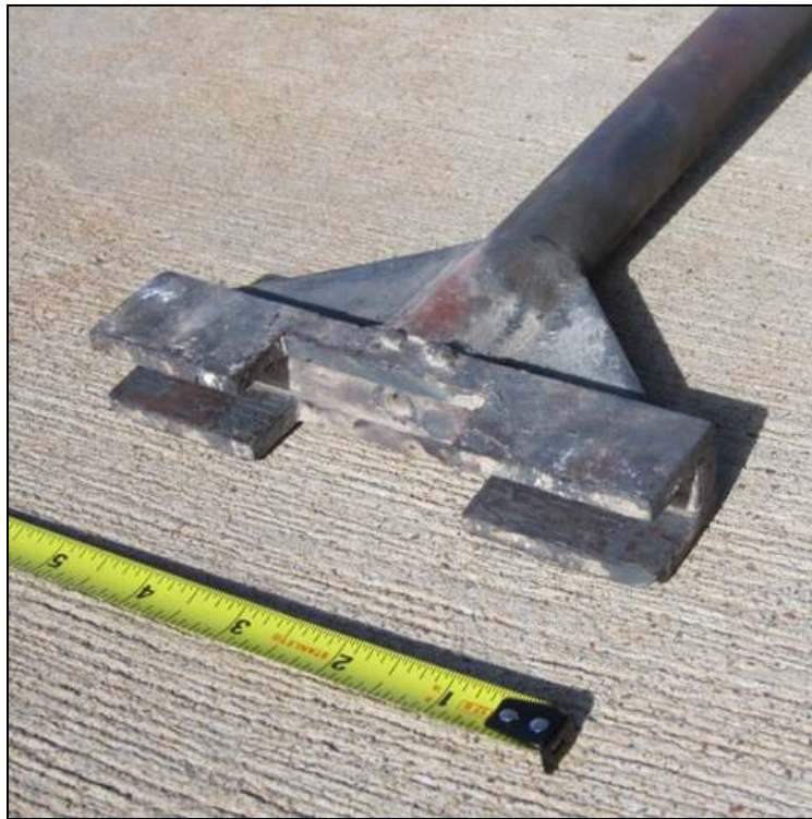
Figure 16: Bottom of agitator rod displaying piece that fits over scraper rod.
