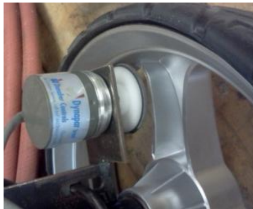
Figure 3. Optical encoder used to calculate speed mounted on the front wheel
