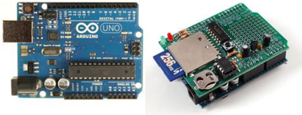
Figure 5. Arduino UNO board, and Arduino Data Logging Shield, used to log data from the sensors into an SD card.
