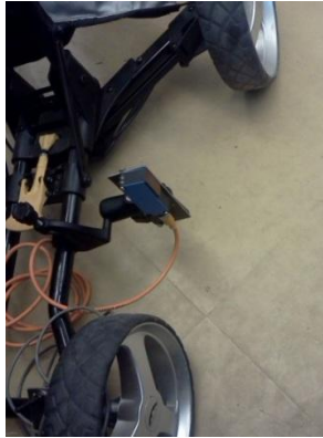
Figure 8. Photoelectric sensor mounted on one side of the cart
