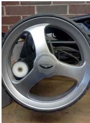
Figure 9. Roller of the encoder making contact with front wheel
