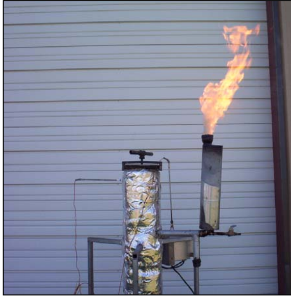
Figure V-2 Photograph of the gasifier and the flare
