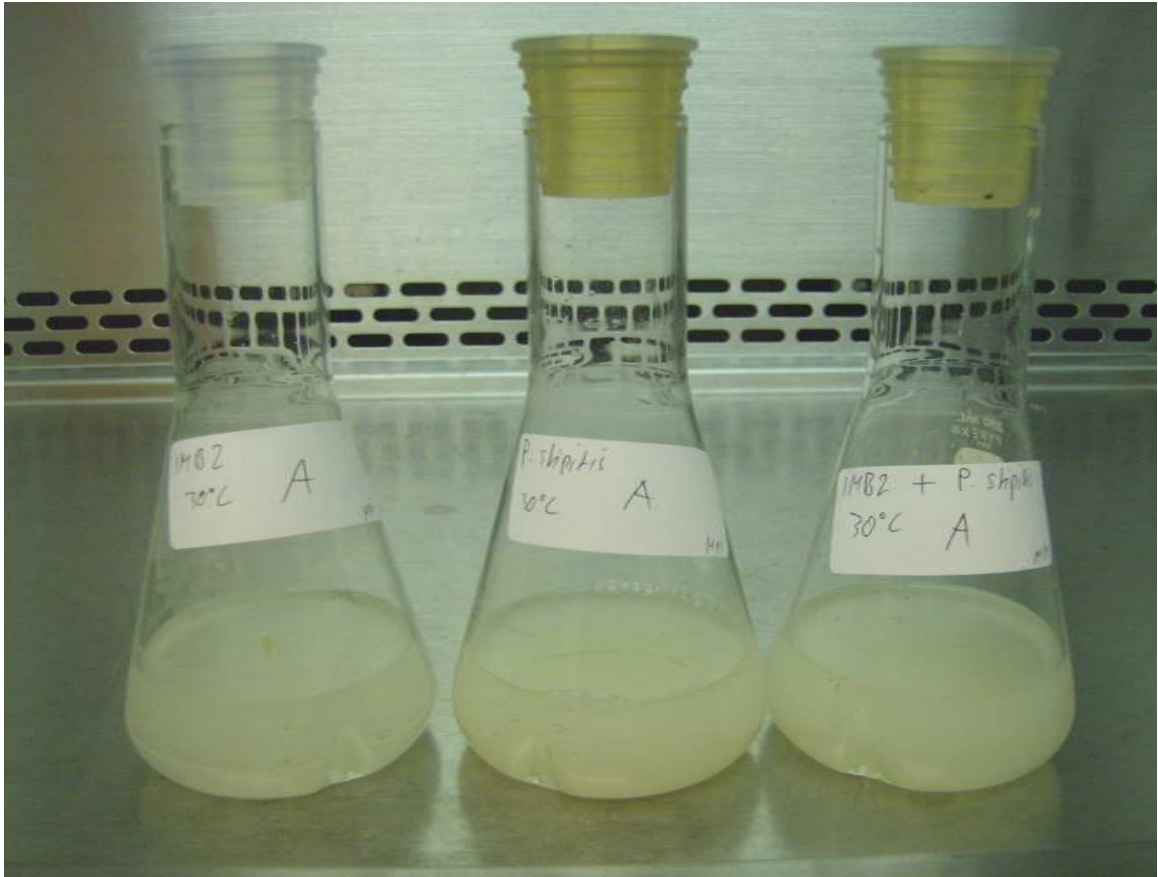
Figure 6: Baffled flasks with stoppers with filter to allow air exchange. Here are the three different cultures for co-culture fermentation.
