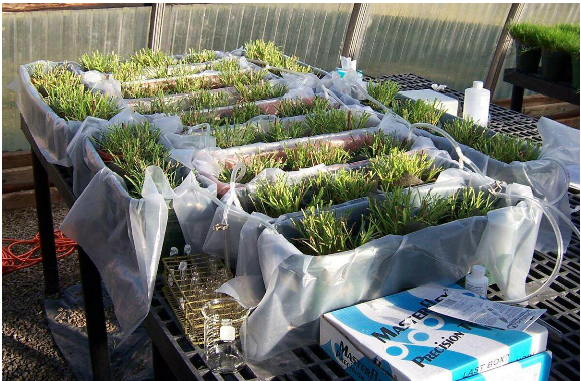
Figure III-a. Photo of actual experiment setup. Border trays limited edge effects of experiment design. Air pump and tubes maintained aeration of hydroponic solution.
