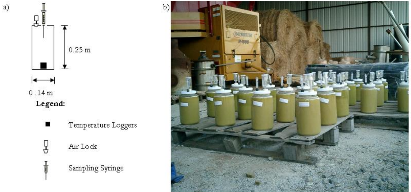
Figure 3.2. Fermentation vessel (3.8-L) setup: a) Schematic representation, and b) Ambient temperature fermentation
