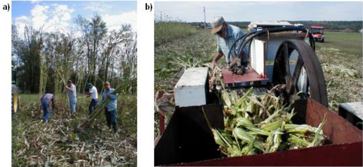
Figure 3.1. Pretreatment of sweet sorghum stalks at Kerr Center a) Manual harvesting, and b) Mechanical pressing using roller press
