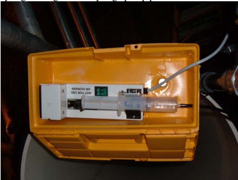
Figure 14: Top view of syringe pump mounted and operating in the toolbox
