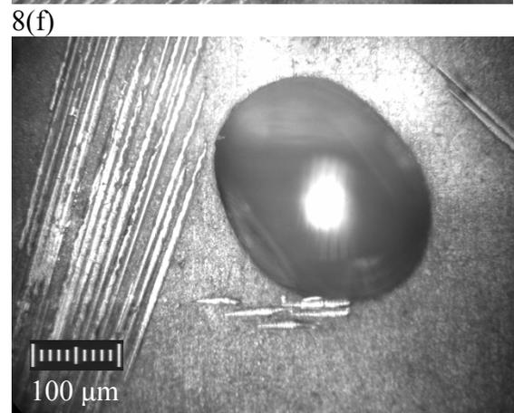
**Figure 5.8: Representative microscopic images obtained at 200x magnifications from the through-the-thickness view (left column), and planar view (right column) samples of the RTM composite molded without post-fill pressure at 17.5% fiber content.**
