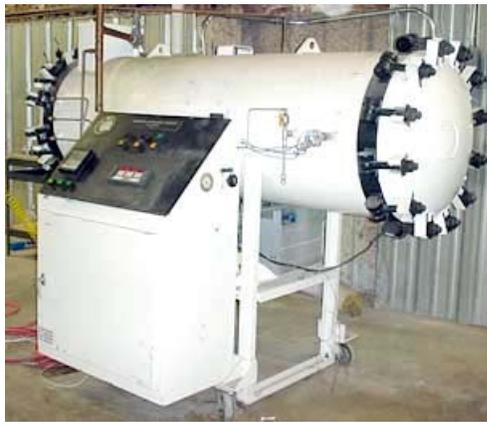
**Figure 1.6: Example of a small autoclave.**
