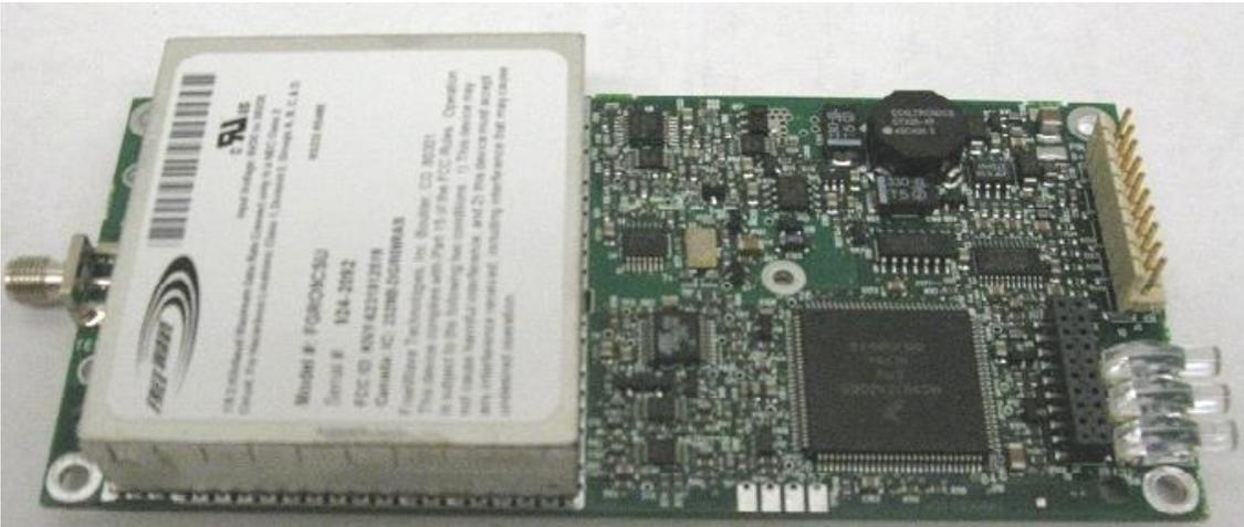
**Figure 11 Freewave OEM Spread Spectrum Radio (900MHz or 2.4 GHz)**
