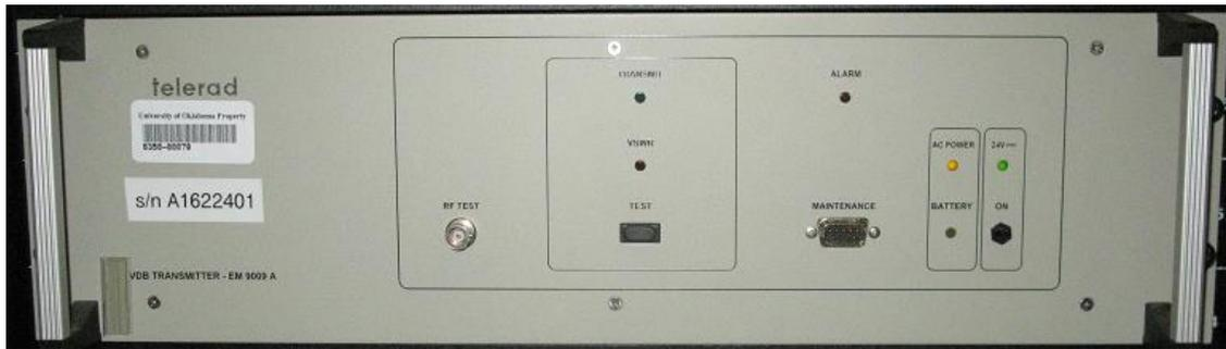
**Figure 13 Telerad (EM9009 A) VDB Transmitter**
