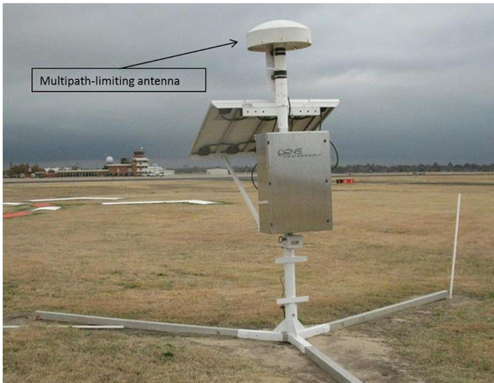
**Figure 9 LAAS Reference Station with Multipath-Limiting Antenna**
