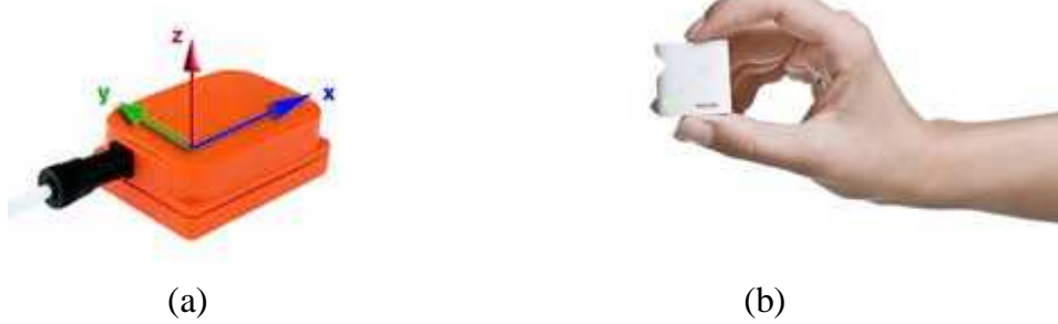
Figure 2.1: Two examples of inertial sensors: (a) MTw sensor from Xsens, US [4]; (b) NWS sensor from Philips, US [5].
