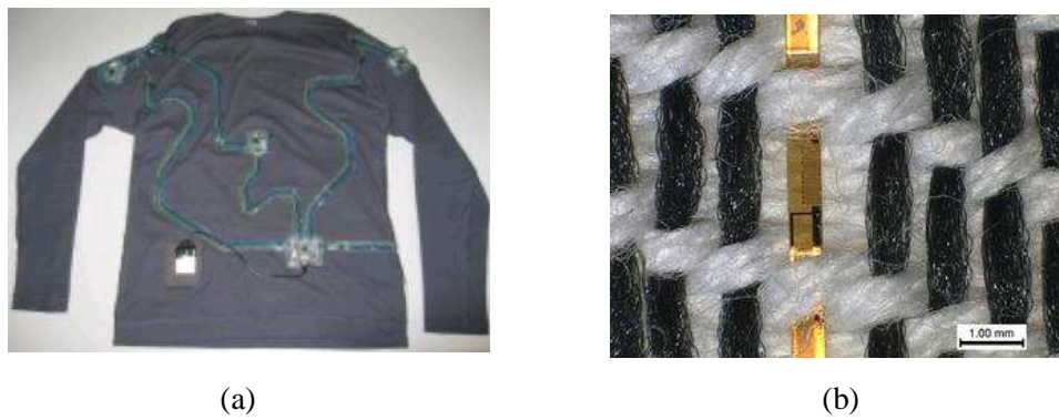
Figure 2.2: Two examples of smart textiles and clothing from ETH, Zurich [6]: (a) SMASH shirt; (b) a woven temperature sensor inserted into a textile.
