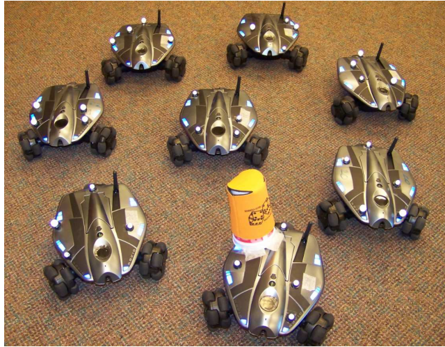
Figure 5.11: Seven Rovio prey mobile sensors and one Rovio predator robot (marked with a yellow cup) are used in the experiment.
