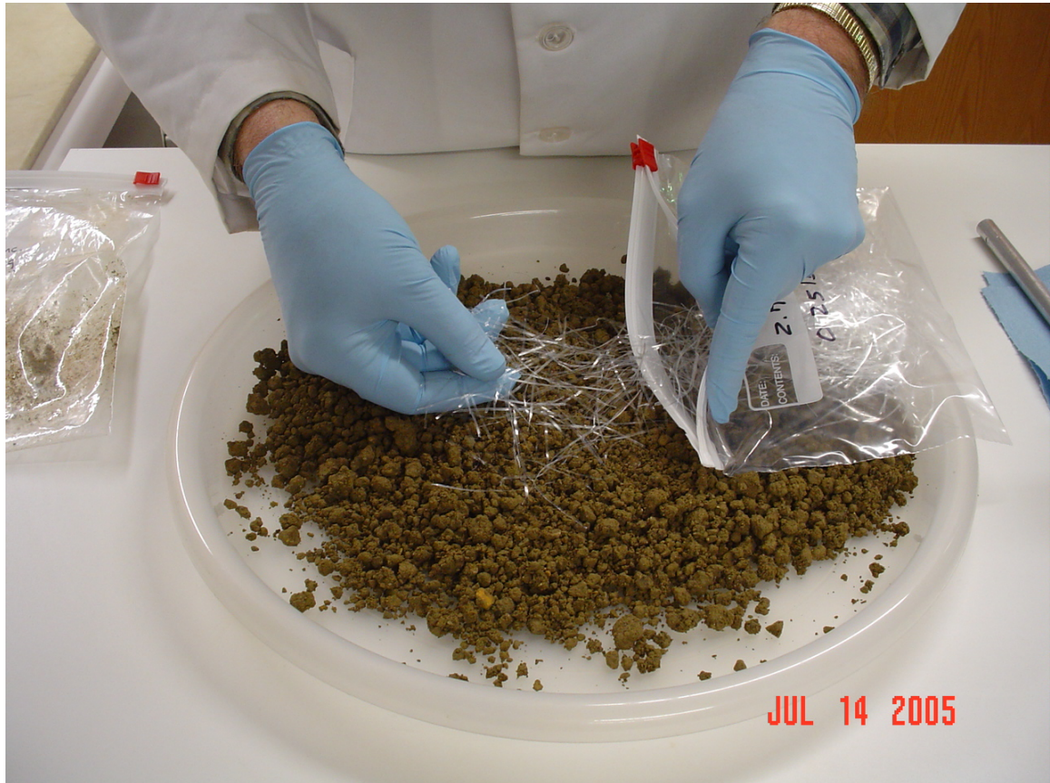
Figure 10. Spreading Fibers over Hydrated Clay Soil Specimen
