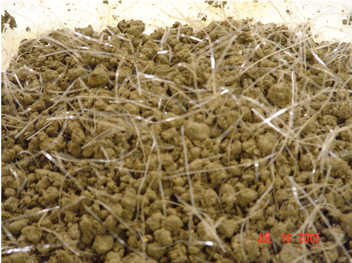
Figure 13. Mixed FRS Specimen Ready for Storage or Compaction
