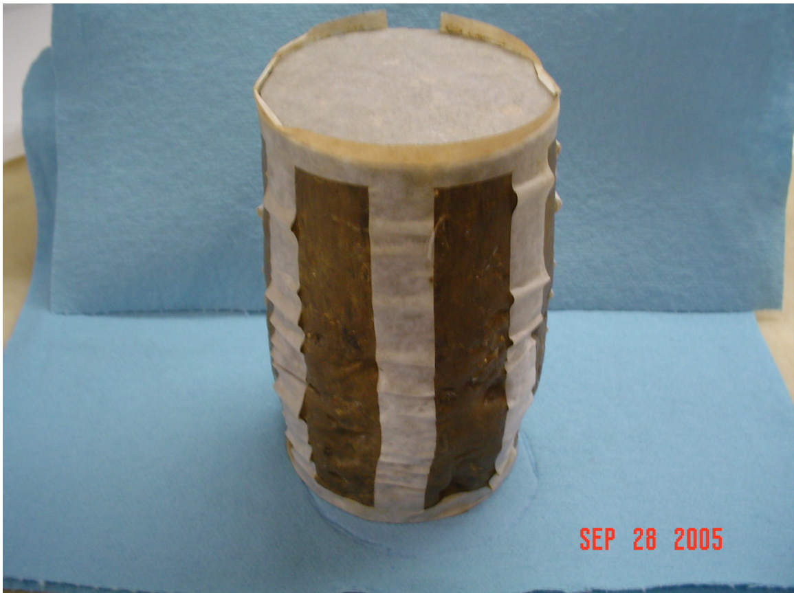
Figure 30. Clay Triaxial Specimen Following Test
