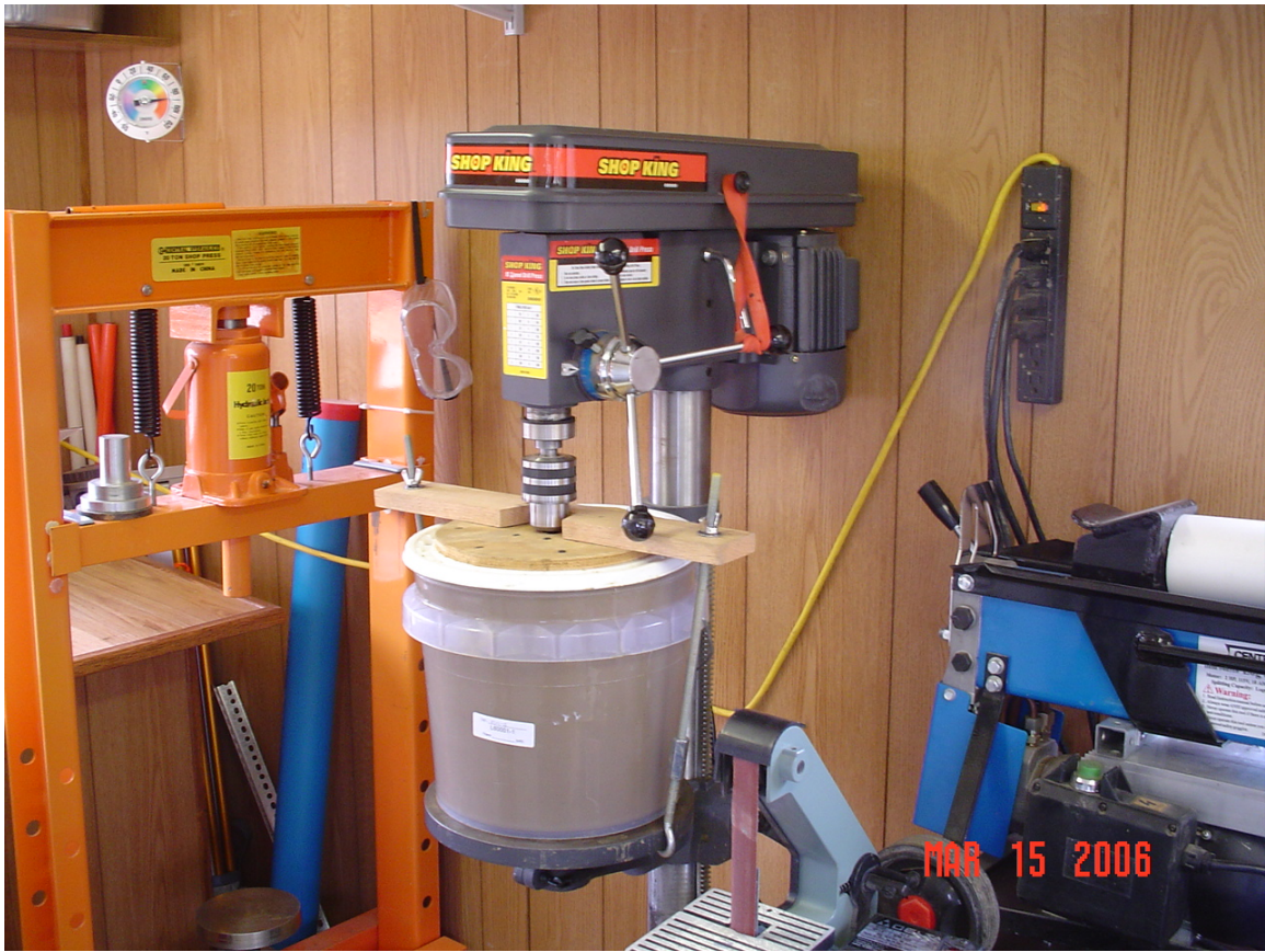
Figure 53. Mixer for Processing Fiber-Soil Specimen Into Slurry
