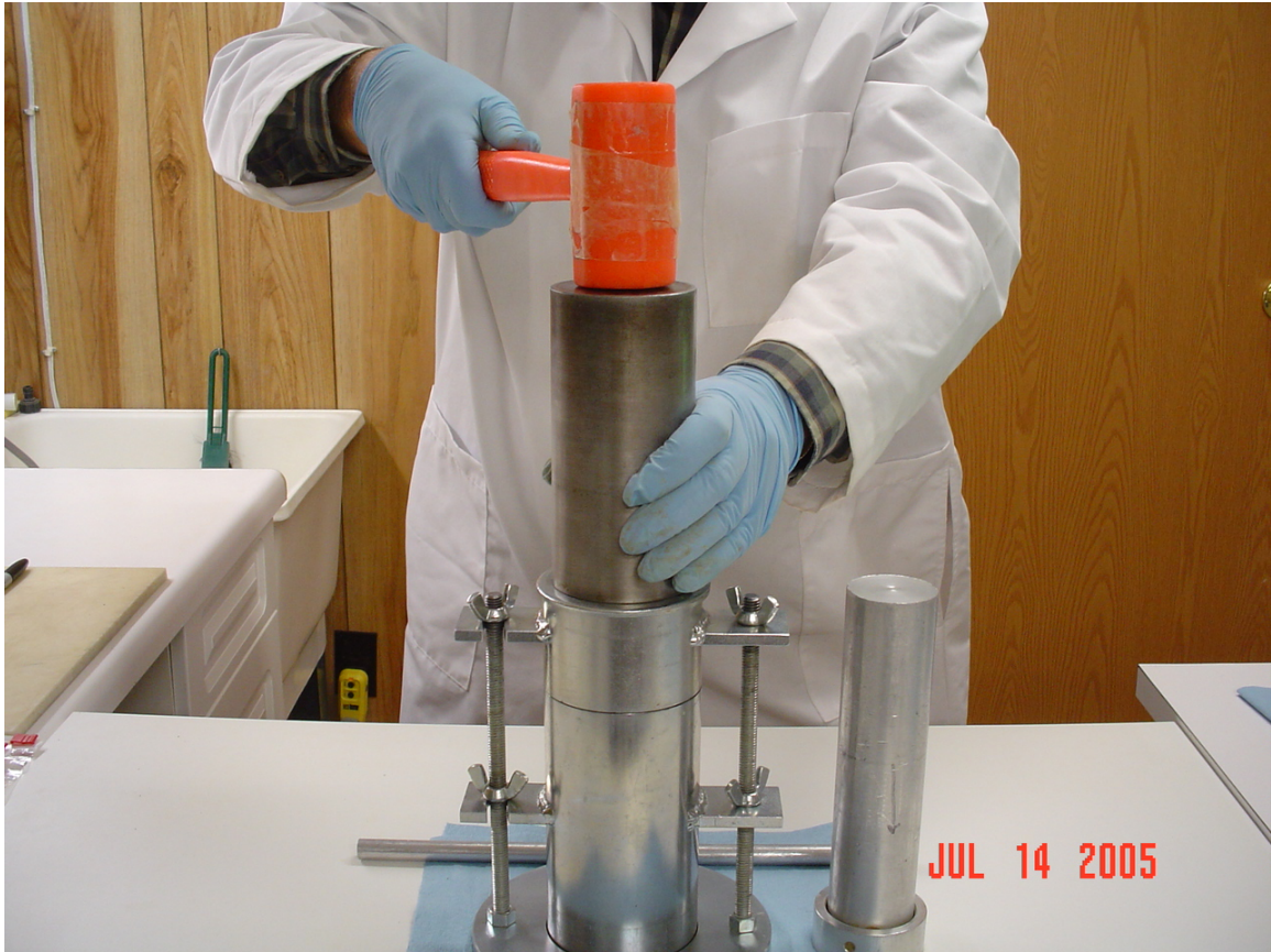
Figure 17. Finishing Compaction with Piston and Guide Ring
