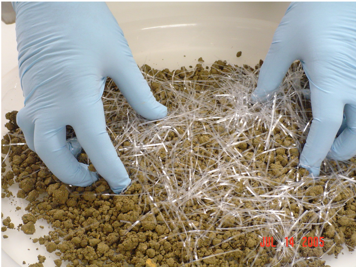
Figure 11. Initial Hand Mixing of FRS Specimen
