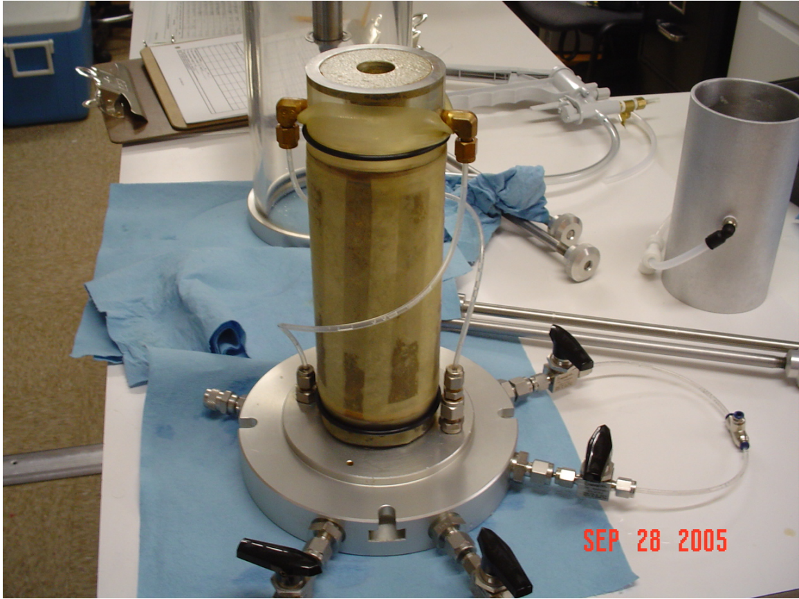
Figure 26. Specimen With Membrane and Top Cap in Place
