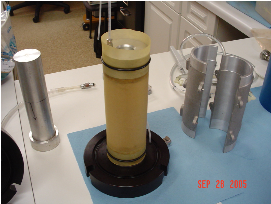
Figure 23. Compacted Sand Specimen After Removal of Split Mold
