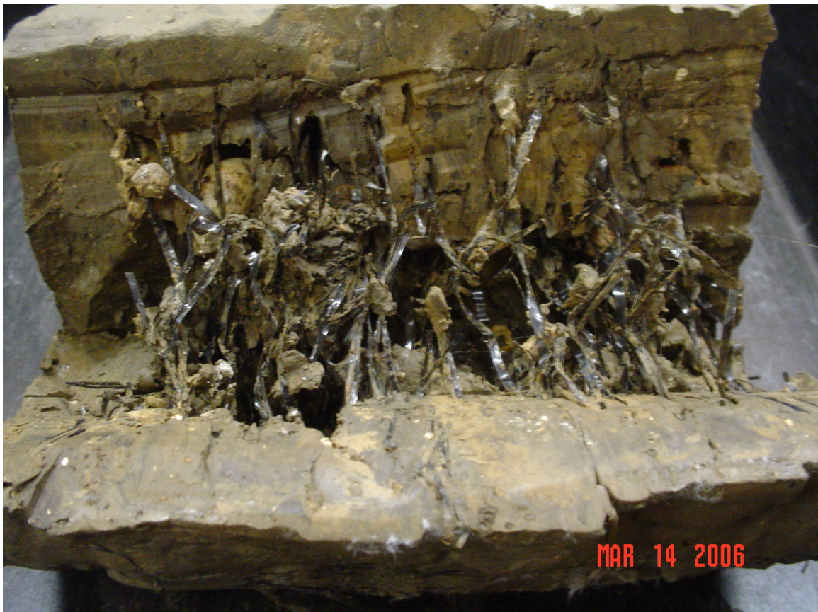
Figure 52. Dissected Field Specimen Following Triaxial Test
