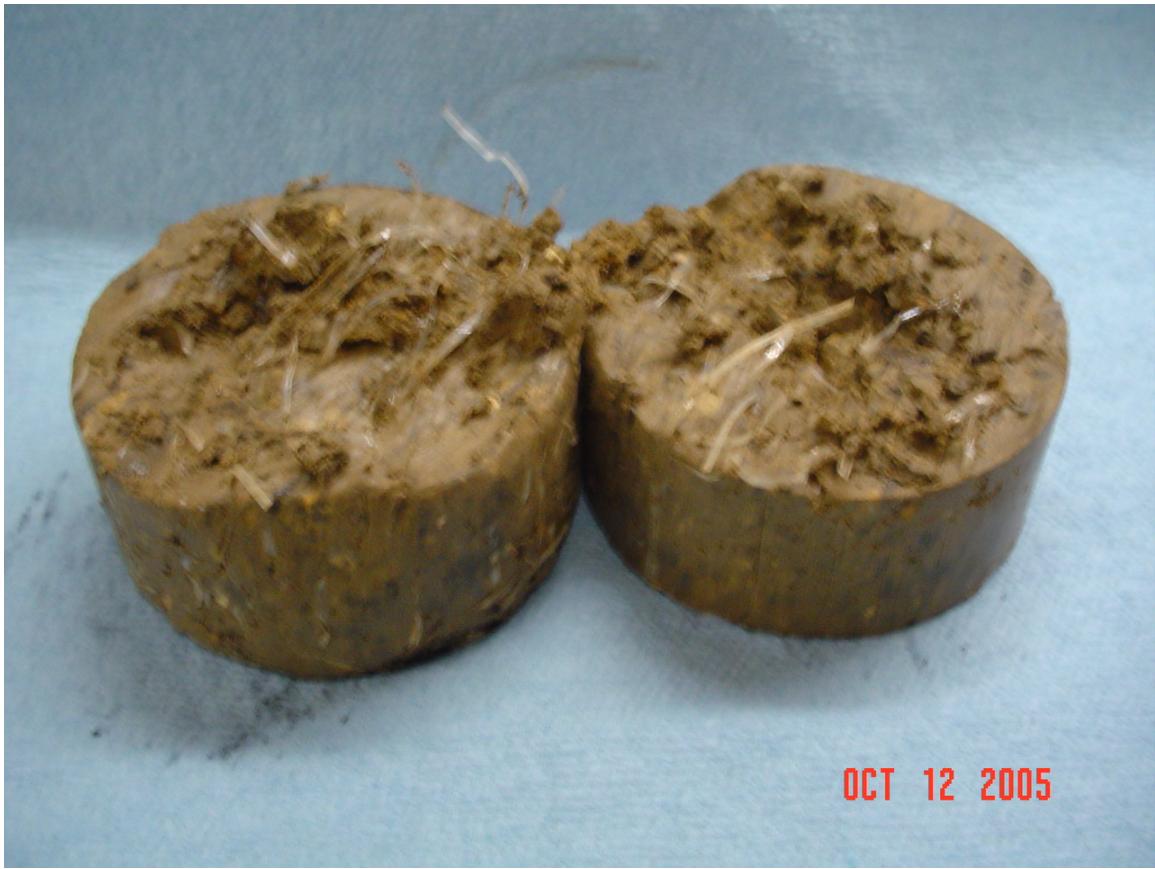
Figure 34. Dissected Direct Shear Clay Specimen With Exposed Fibers
