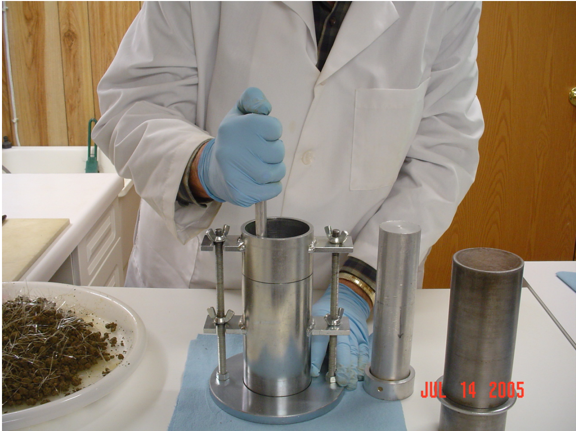
Figure 16. Rod Plunged to Near Bottom of Mold During Initial Compaction
