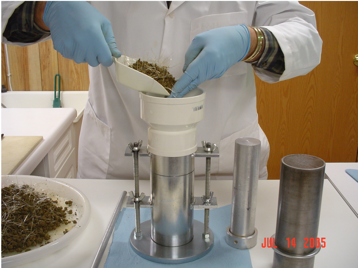
Figure 14. Placement of Loose Specimen into Mold
