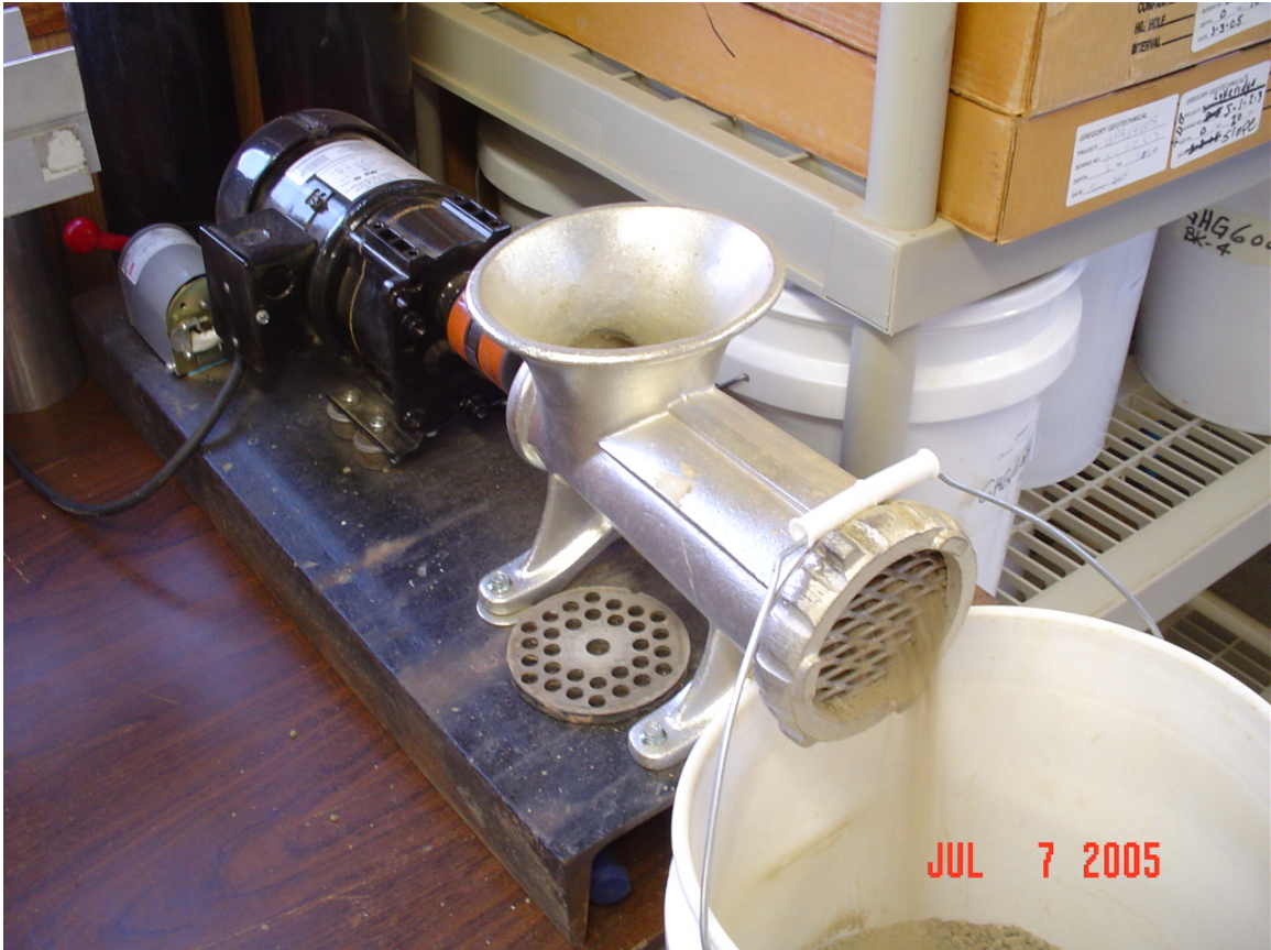
Figure 8. Processing of Clay Sample
