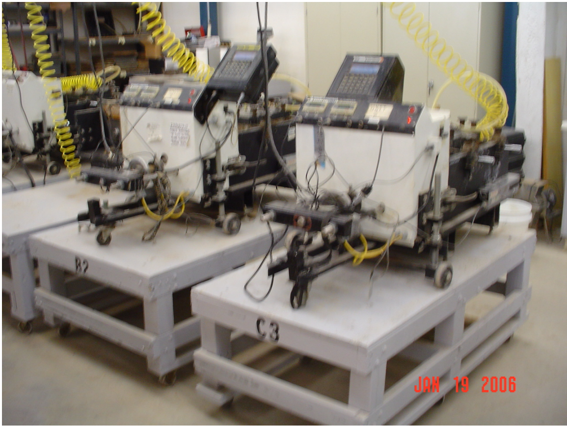
Figure 39. Large Scale Direct Shear Machines Used in Interface Tests
