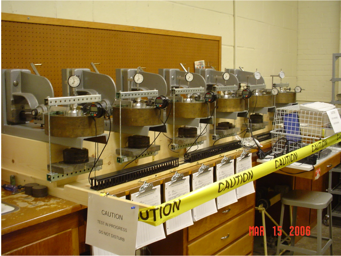
Figure 35. Direct Shear Creep Devices
