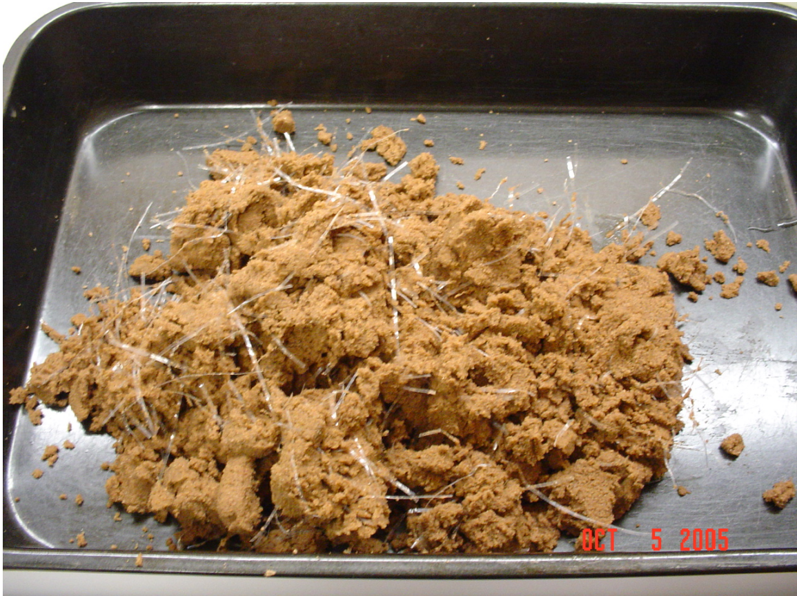
Figure 1. FRS Mixture with Sand
