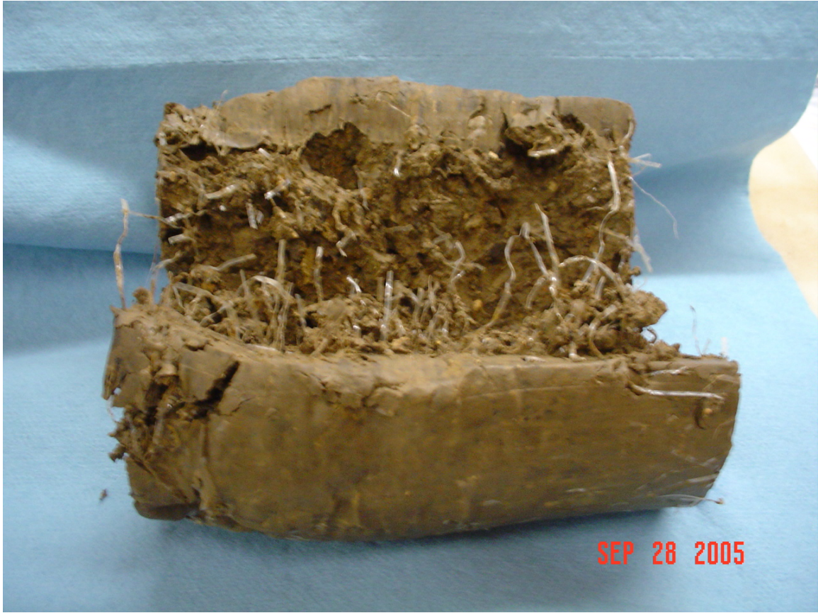
Figure 31. Dissected Triaxial Clay Specimen With Exposed Fibers
