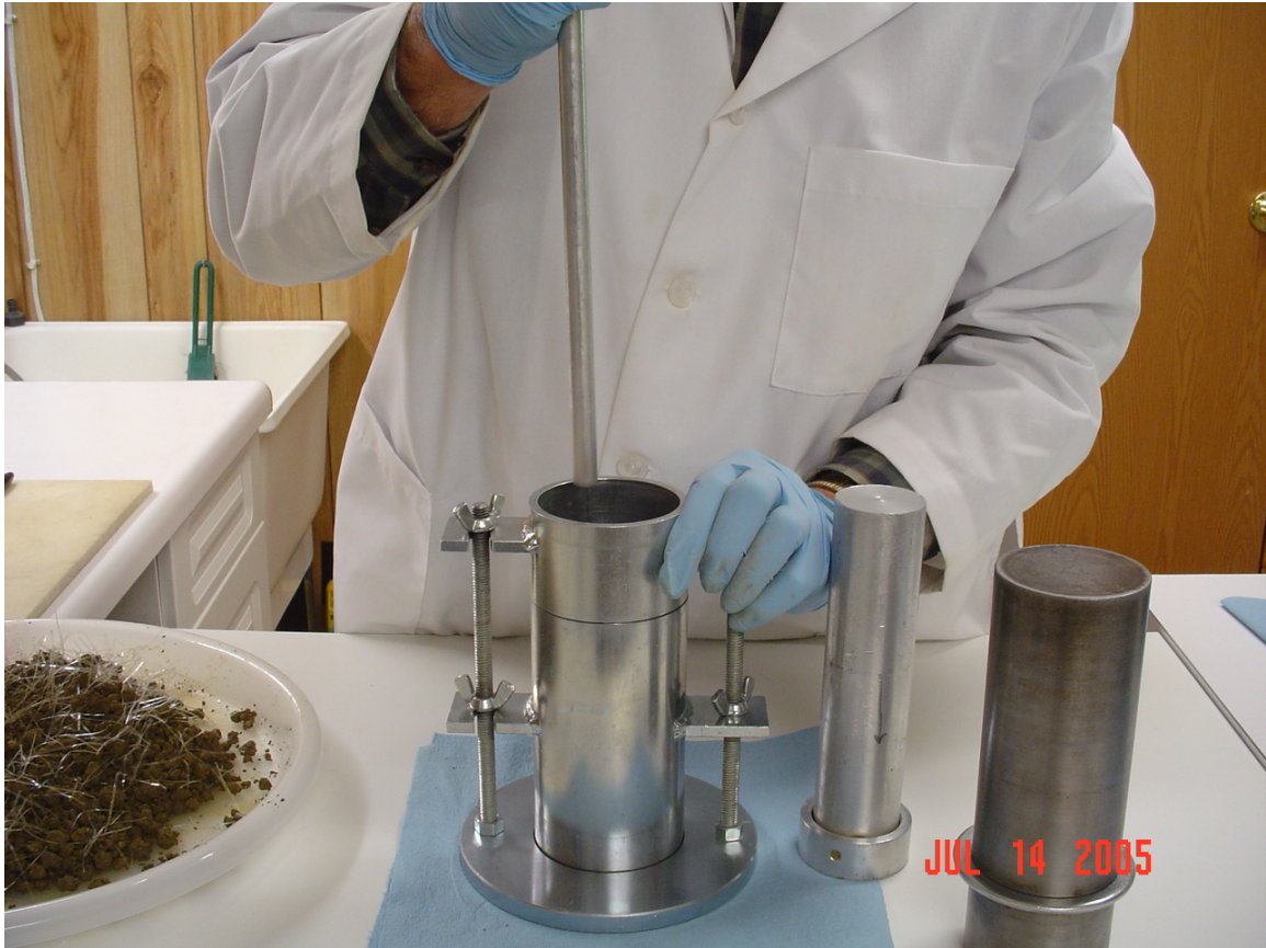
Figure 15. Compaction with Metal Rod
