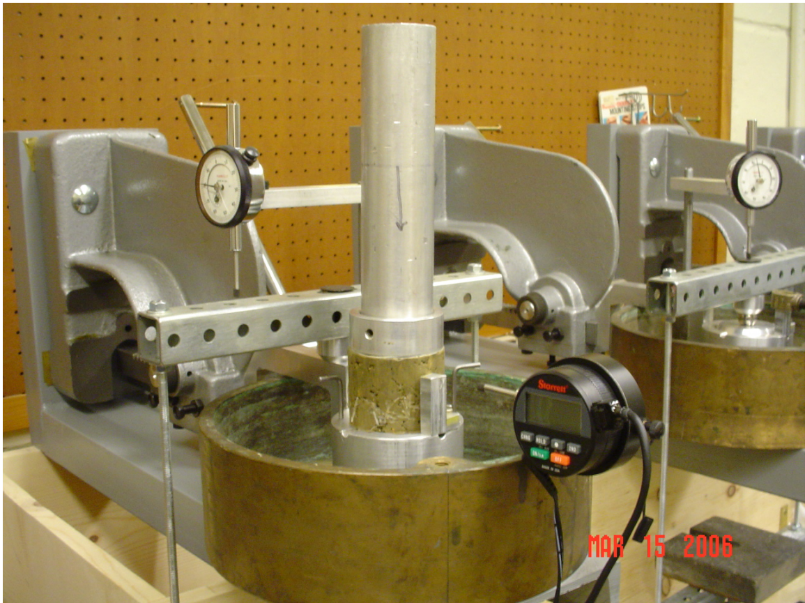
Figure 36. Mounting Clay Specimen in Creep Device
