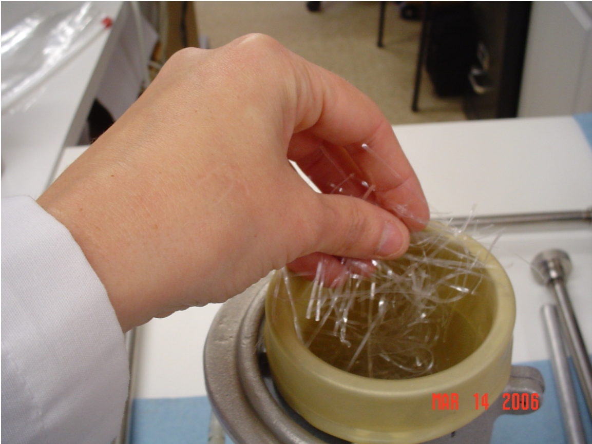
Figure 22. Addition of Fibers to Sand Specimen During Compaction
