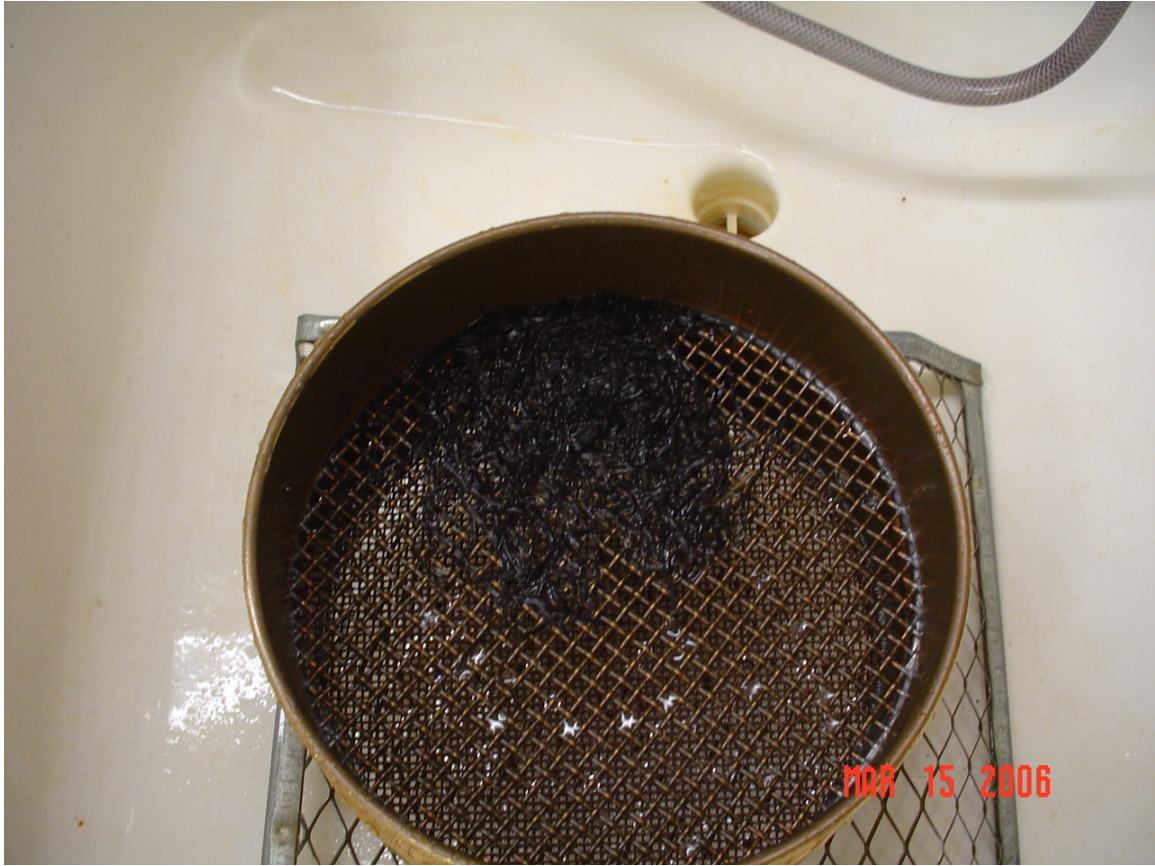
Figure 54. Sieving of Slurry to Extract Fibers
