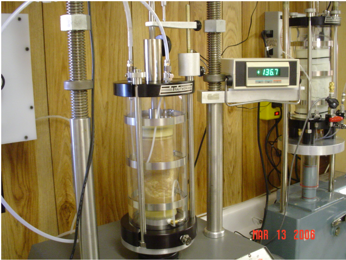
Figure 38. Triaxial Test on Sand Specimen
