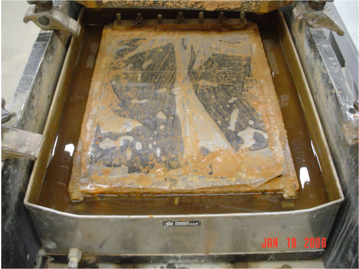
Figure 41. Sheet Material on Bottom Shear Box After Interface Test
