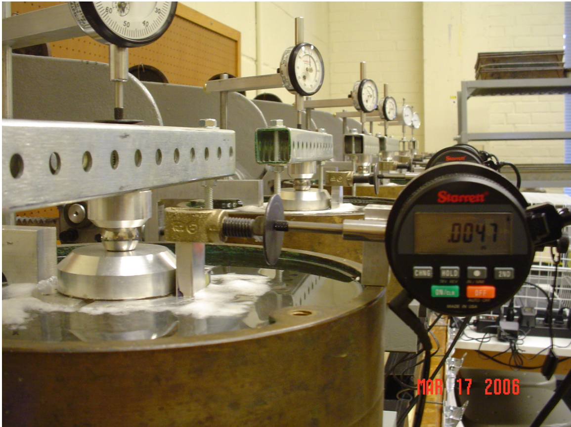
Figure 37. Fully-Mounted Creep Specimen With Water in Reservoir
