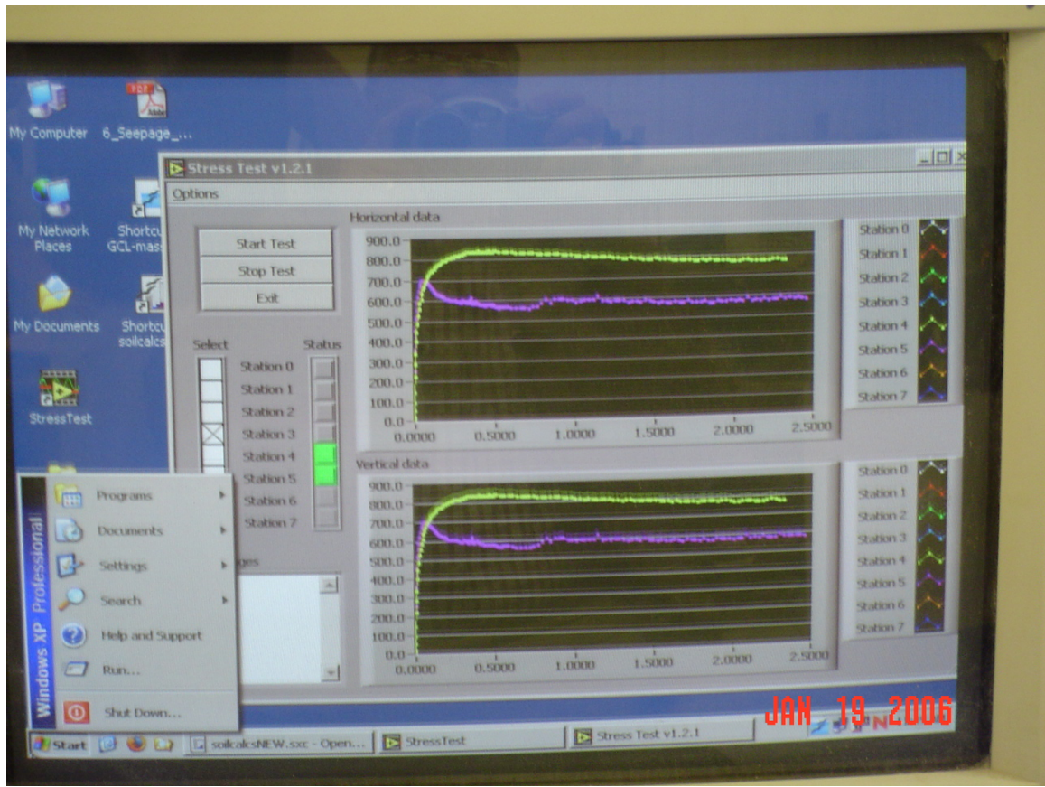
Figure 40. Real Time Data From Interface Shear Tests (Green = Sand, Purple = Clay)
