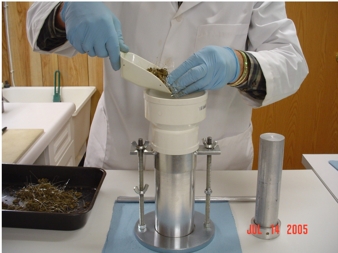
Figure 18. Preparation for Compaction of Direct Shear Specimen
