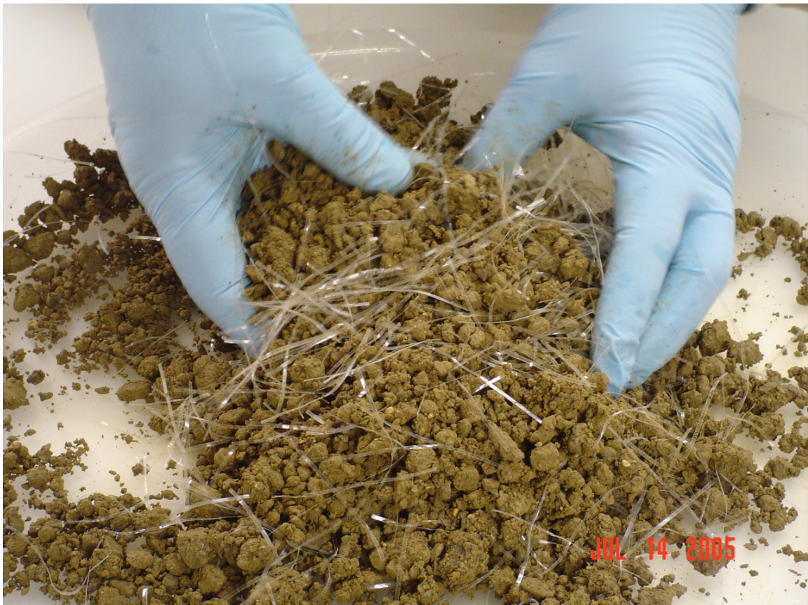
Figure 12. Final Hand Mixing of FRS Specimen
