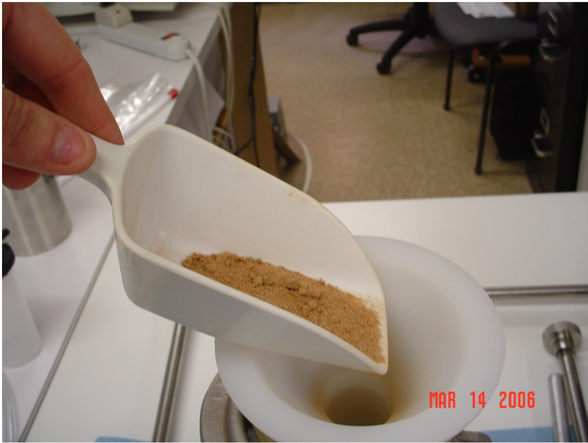
Figure 21. Preparation of Sand Specimen in Split Mold
