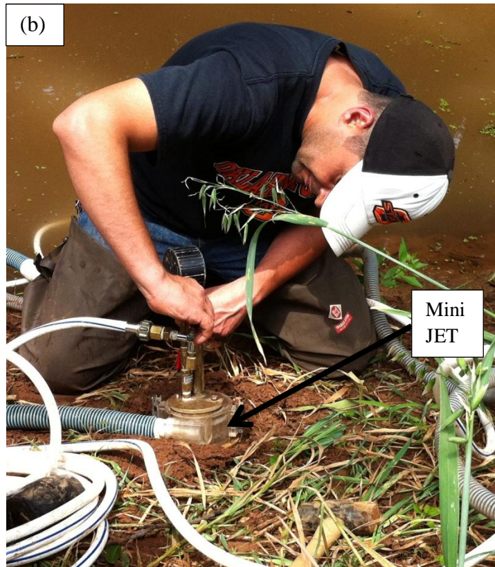
Figure 6.5. (a) Location of the reaches in Cow Creek and (b) In – situ “mini” JET device.
