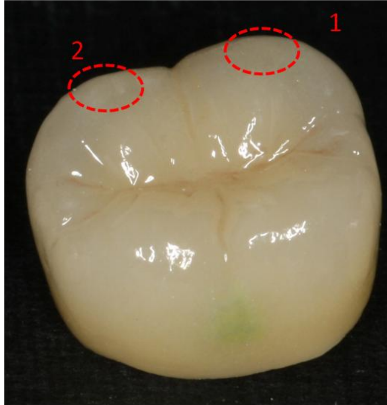
Fig.7-1 Nanoindentation were performed on the two cusp indicated to obtain residual stress difference
