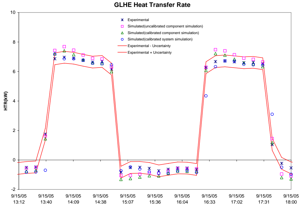
Figure 5.7 GLHE heat transfer (rejection) rates for five hours of a typical cooling day.
