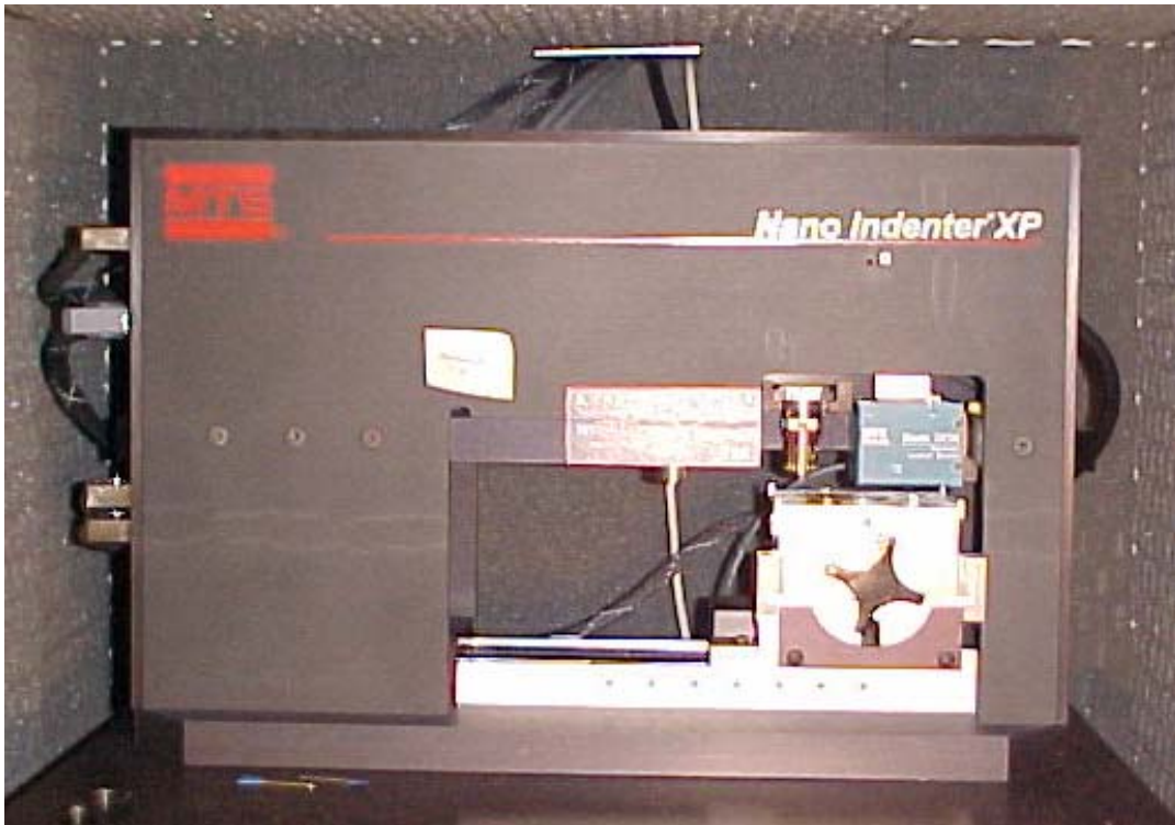
Figure 4.10: MTS Nano Indenter XP System
