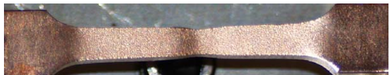
Figure 5.2 : Photographs of the deformation of the polycrystalline copper (C11000) under tensile loading
