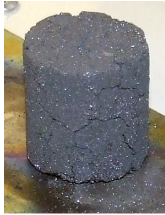
(b) Coarse metal reinforcement led to cracking of the pellet.
