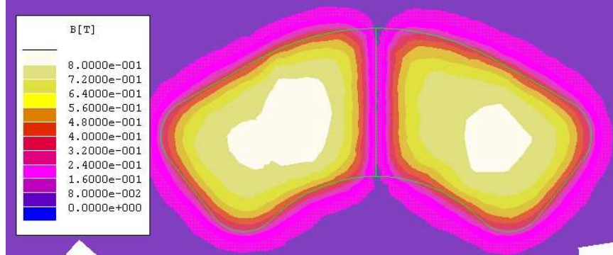
Figure 2.7: Magnetic circuit air gap flux density (FEM results)
