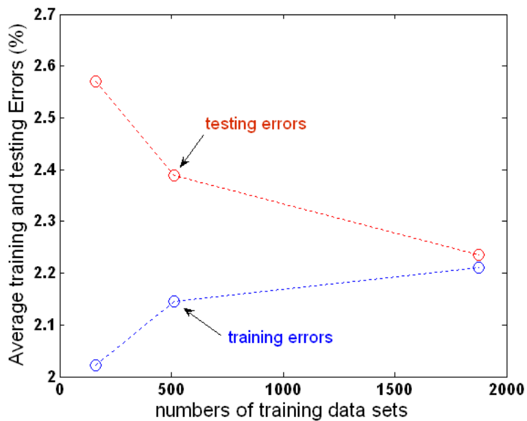
Figure 6.79 Training and Testing Errors for ANFIS-SC MRR Models
