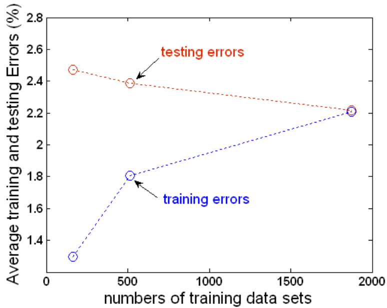
Figure 6.78 Training and Testing Errors for ANFIS-GP MRR Models
