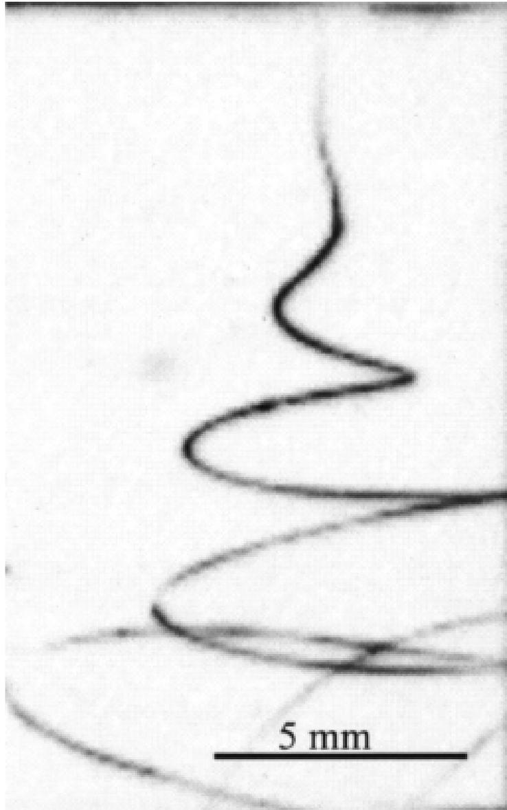
Figure 1-3 Bending instability (Yarin et al., 2001).
