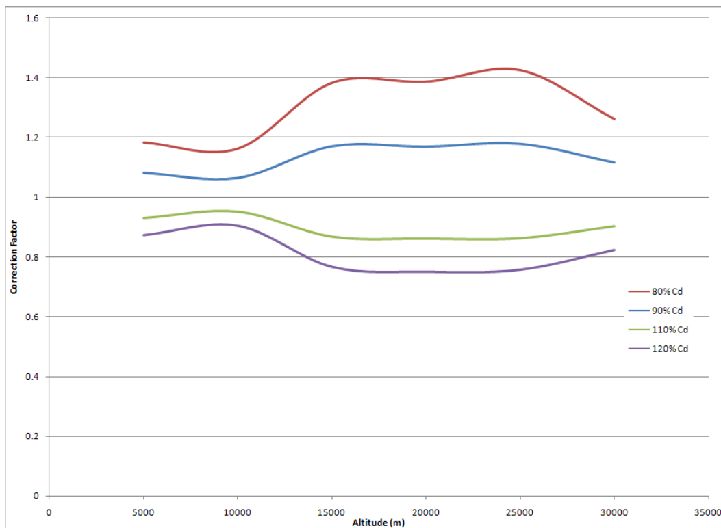
Figure 32 Variation of Correction Factors as Function of Altitude for the varying Cd
