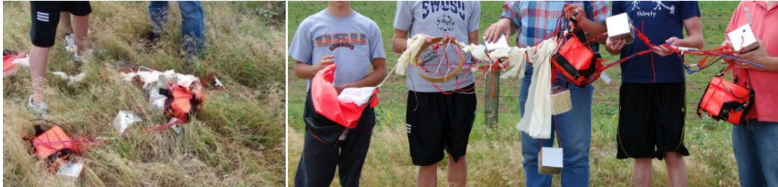
Figure 9 Balloon Fouling Damage (ASTRO-14)
