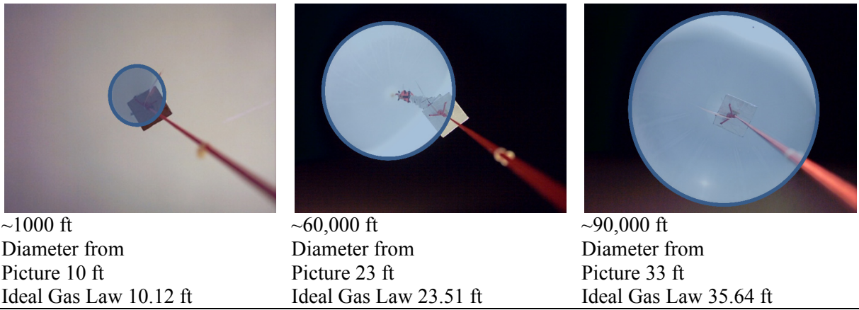
Figure 7 Expansion of Balloon during ASTRO-04
