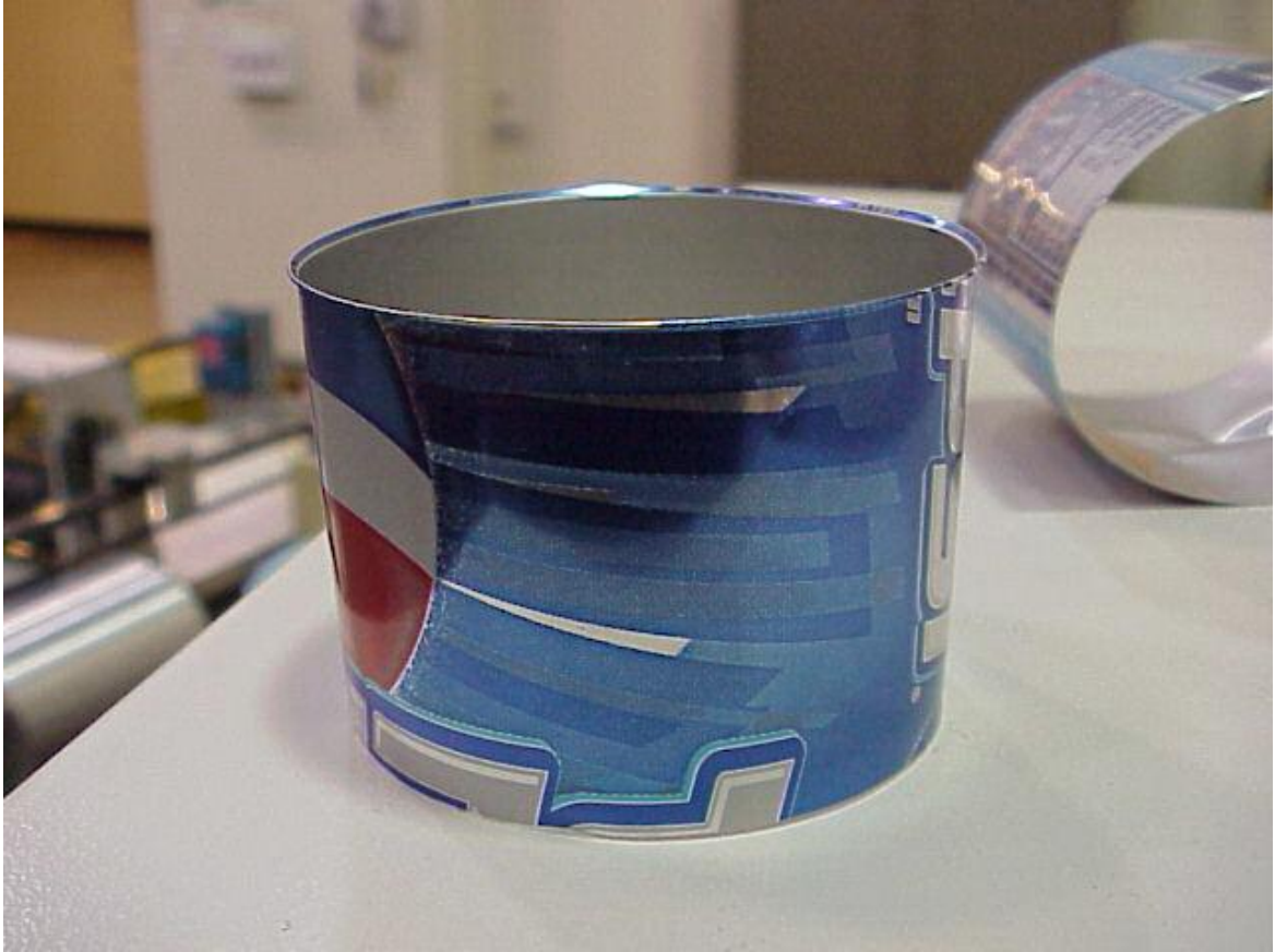
Figure 42 – Buckling at Outer Edge of Shell
