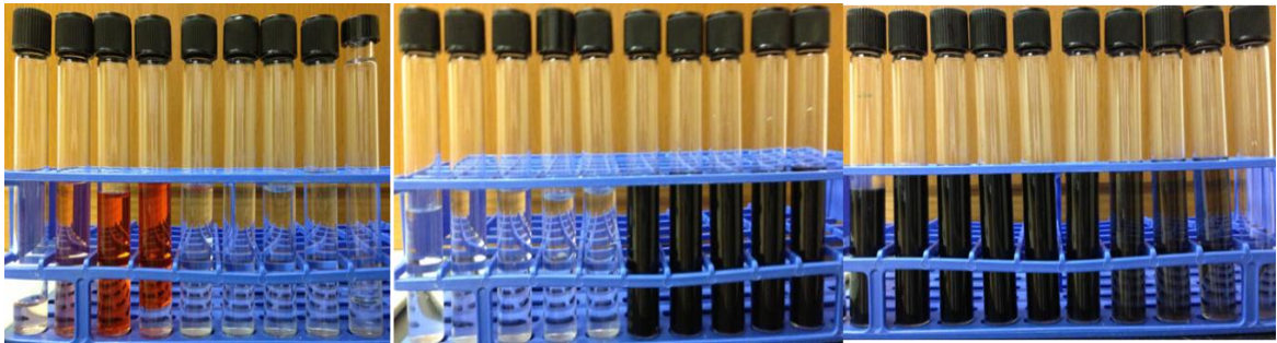
Figure 1- 42: SO 3 -MWNT dispersion injection in the presence of oil phase.
