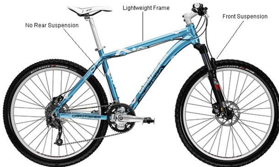
Figure 1. Gary Fisher Tassajara – Example of a Hardtail Mountain Bike (photo used with permission)
