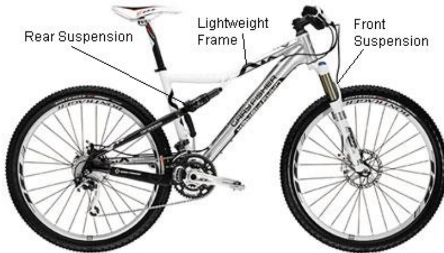
Figure 2. Gary Fisher Supercal – Example of a Full Suspension Mountain Bike (photo used with permission)
