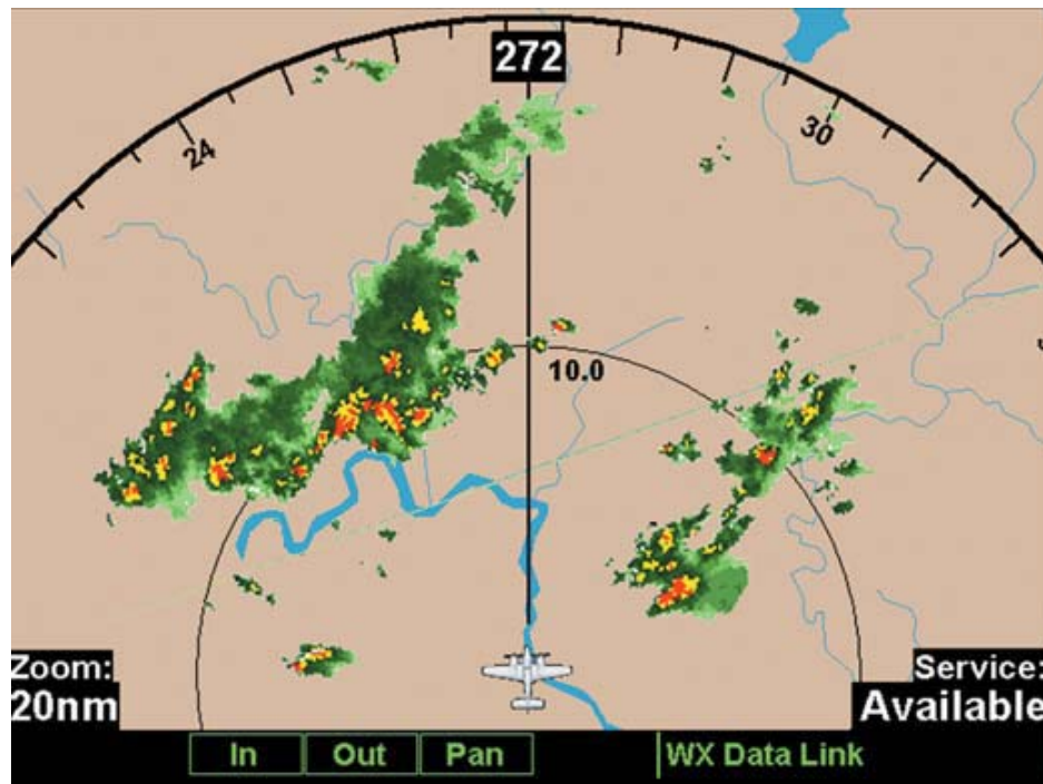
Figure 4. Sample CDTI Display including Weather. (ADS-B Aviation Rulemaking Committee, 2008, p.D-7)
