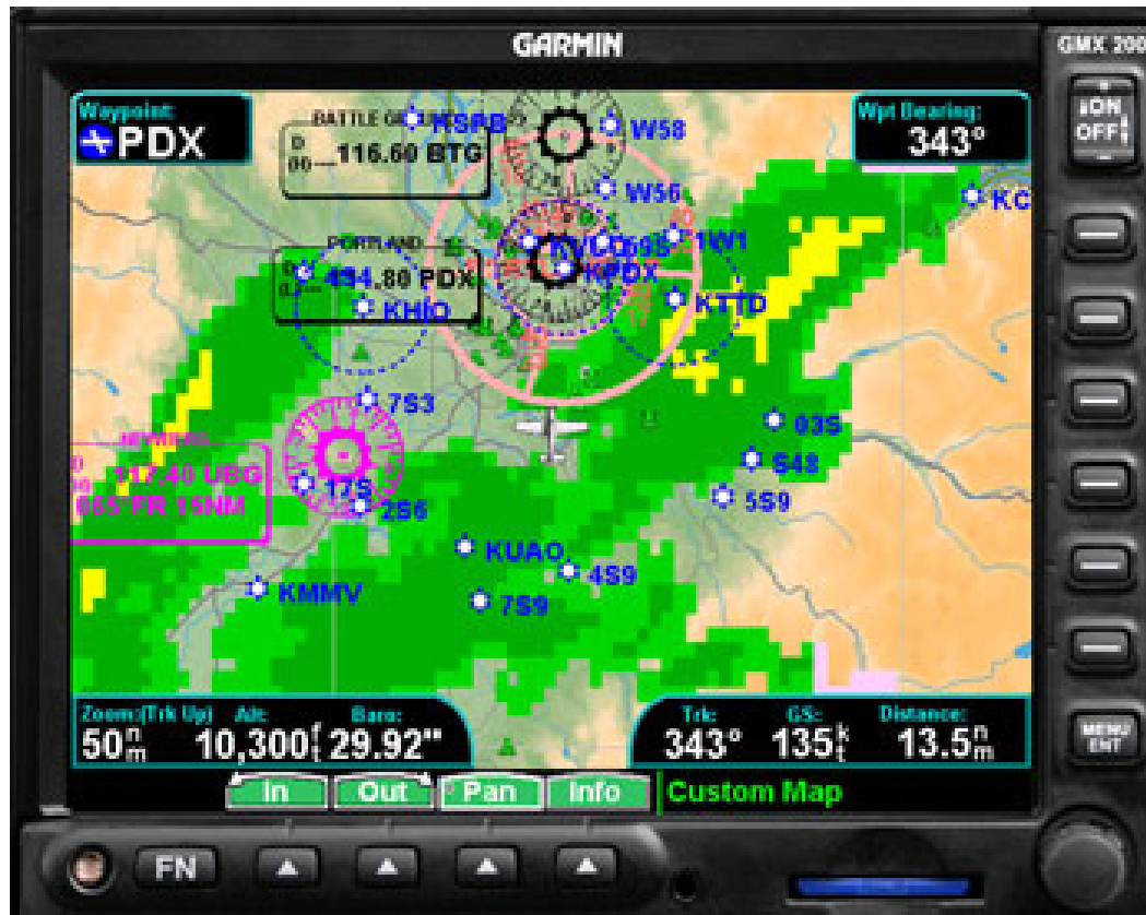
Figure 5. Sample Garmin ADS-B cockpit display including traffic and weather (Flt Tech Online, 2009).
