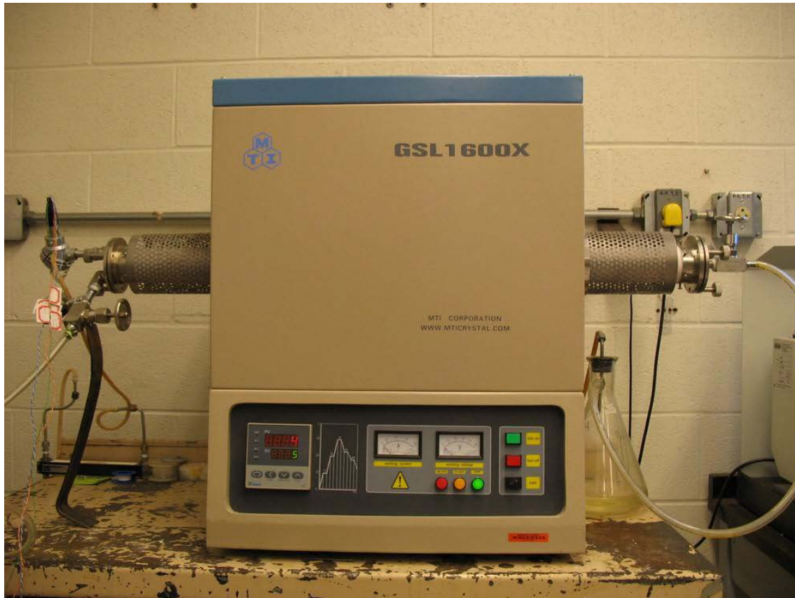
Figure F.1 Optical image of the tube furnace for sintering process. Processing gas flows in through the inlet on the left of the horizontal tube, and exits through the outlet on the right. A high purity (>99.8%) alumina tube is used for this furnace.
