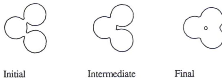
Figure 2.17 Illustration of the densification of three adjacent particles. 37
