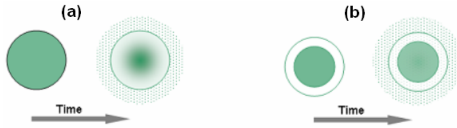
Figure 2.8. Schematic diagram of the diffusion controlled system: (a) matrix system and (b) reservoir system
