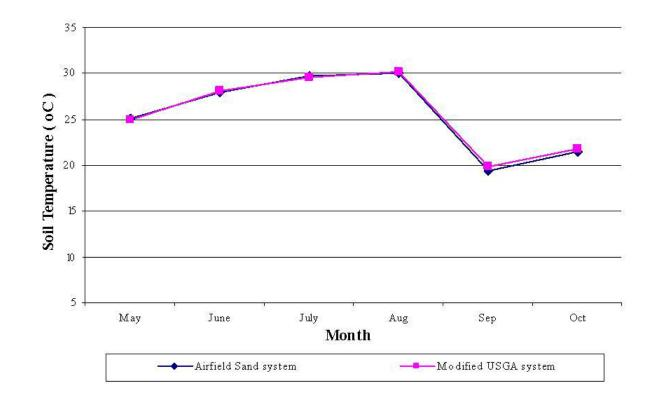
Figure 25. The monthly canopy temperature changes in Airfield and Modified USGA sand systems.
