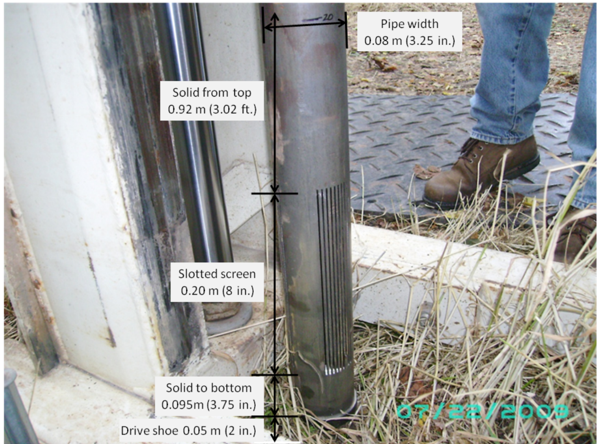
Figure 1.1 Slotted section of gravel permeameter in driving position showing alignment of slot and slot-free areas.
