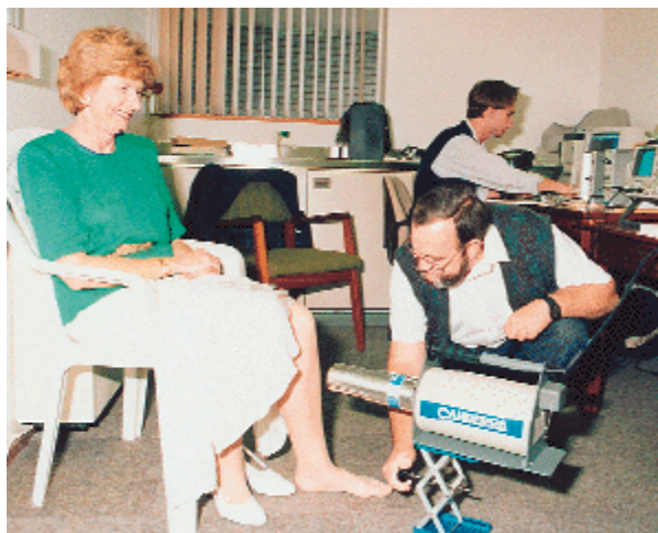
Figure 1. Words Into Action. Andrew Todd Monitors the Spectrum as an Assistant Positions the XRF Machine to Measure Tibial Bone Lead in a Subject.
