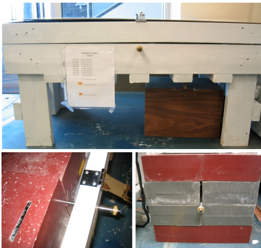
Figure 4.12 Experimental setup for testing the portable system against thorium-enriched epoxy blocks. Above: Wooden box housing the ^{232}\text{Th} -enriched blocks in two rows of four. Bottom left: View of the inside of wooden housing with probe 1 inserted between the two rows of blocks. Bottom right: Blank epoxy blocks with probe 2 inserted in the center.
