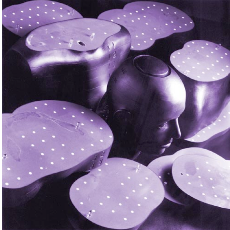
Figure 5.16 Photograph of a partially disassembled Rando ® phantom. Clearly depicted are the grids of plugged holes used for dosimeter placement, as well as the human skeleton. Reproduced with permission of The Phantom Laboratory - www.phantomlab.com .
