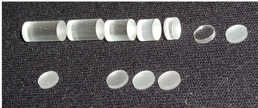
Figure 4.3 Different \alpha - \text{Al}_2\text{O}_3 :C dosimeters investigated for use as radiation sensor on the probe, with thickness varying between 1 mm and 10 mm.
