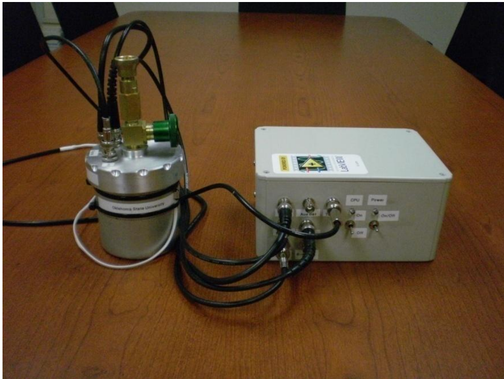
Figure 72. The flight version TEPC connected to the computer box. The box contains the CPU, power supply, battery, high voltage power supply, linear amplifier, and multichannel analyzer.
