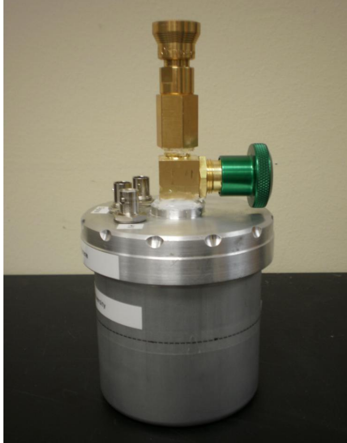
Figure 15. One of the TEPCs fit onto the sealed canisters.
