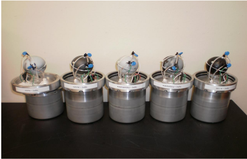
Figure 12. The five proportional counters fabricated for this study. From left to right: Nylon, acrylic, polyethylene, polystyrene and A-150 tissue equivalent plastic.
