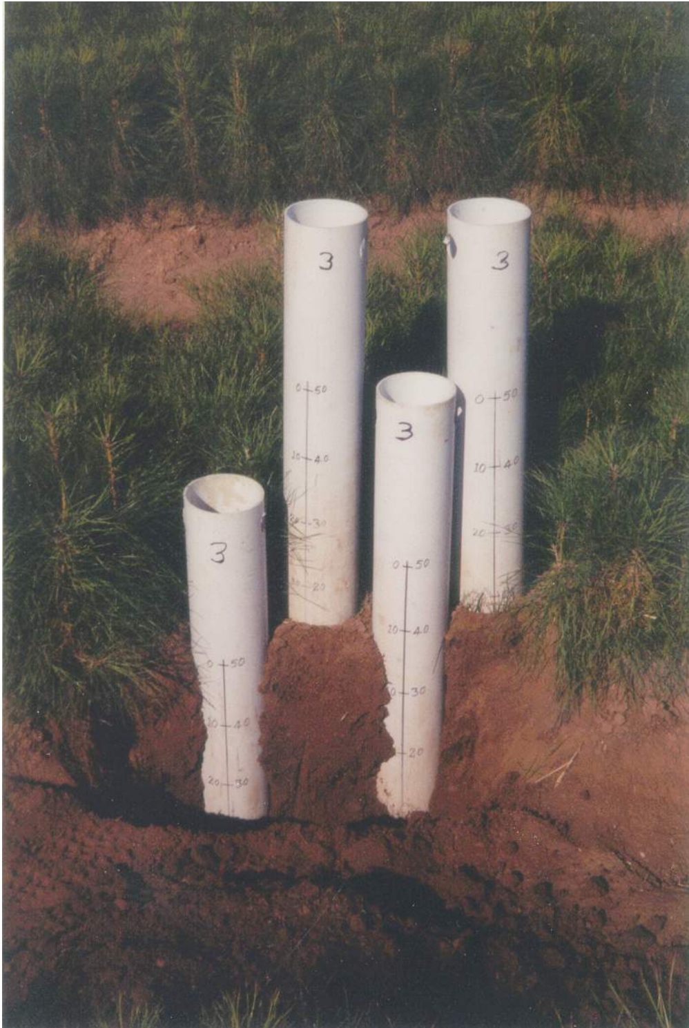
Fig. 3. Collection of seedlings by Insertion of four pipes up to 50 cm.
