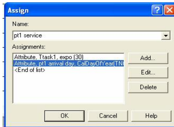
Figure 5.7 Assign Block to set Primary Task Service Time and Track Arrival Day
