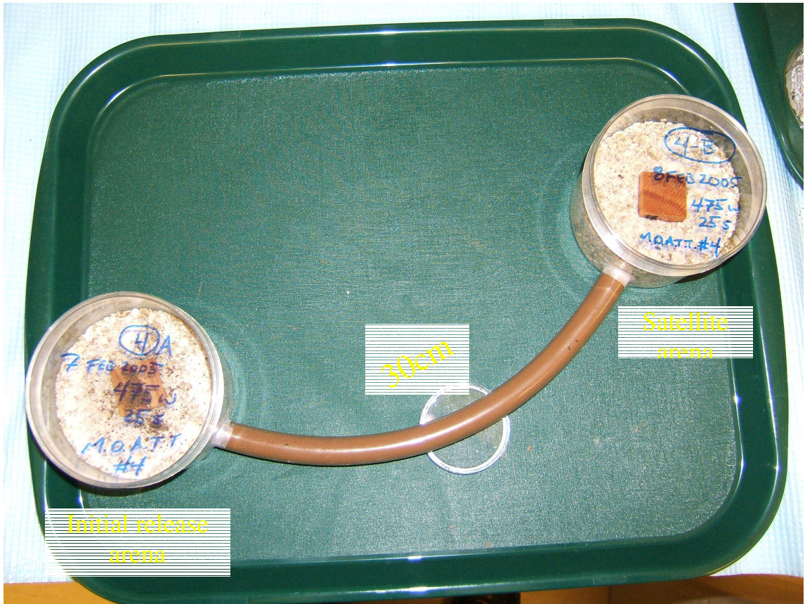
Figure 4.1. No-choice test unit with initial release and satellite arenas containing sand/vermiculite substrate and a pine block, connected by a soil-packed 30cm foraging tube.
