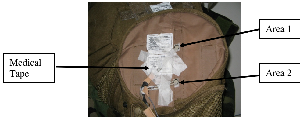
Figure 18. Placement of Localized Pressure Sensor
