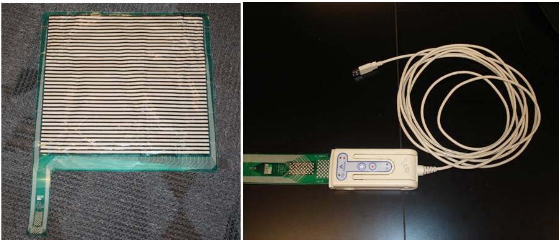
Figure 14. Tekscan BPMS Sensor (# 5350) and Evaluation Sensor Handle
