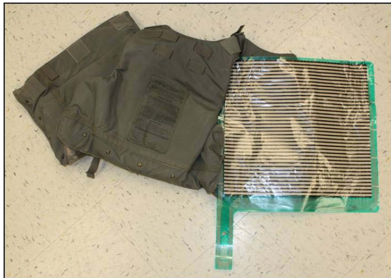
Figure 20. Sensor (# 5350) Attached to the Inner Side of the Left Front Interceptor™ Vest
