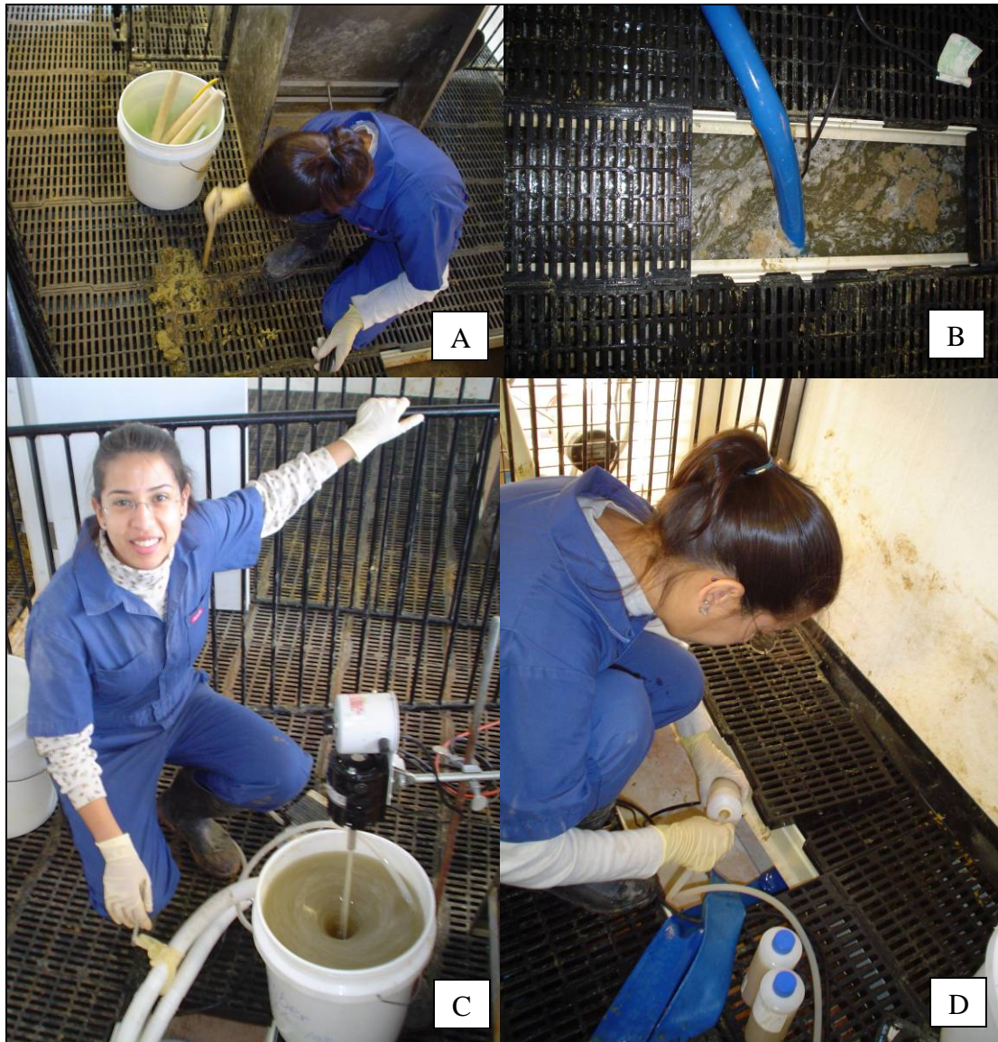
Figure III.2. Pit content sampling: A) Scraping manure on the floor and adding into the pit, B) Mixing pit content with the aid of a recycling submergible pump, C) Homogenizing slurry sample, D) Transferring slurry samples to 500 ml bottles.
