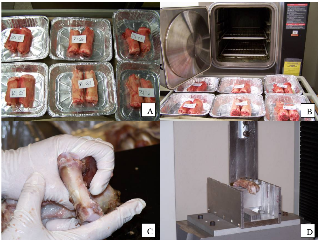
Figure III.3. Bone strength measurement: A) One batch of front feet, B) Batch of feet ready to be placed into the autoclave, C) Metacarpals removed after cooking the feet, D) Metacarpals placed in the base of the Instron instrument.
