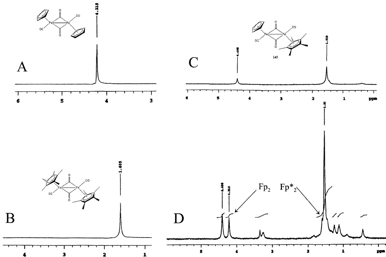
Figure 4.2 300 MHz  $^1\text{H}$  NMR of  $[\text{Cp}(\text{CO})_2\text{Fe}]_2$  (A),  $[\text{Cp}^*(\text{CO})_2\text{Fe}]_2$  (B), 145 (C), and 145 after heating at  $150^\circ\text{C}$  in dioxane under CO (D). (All spectra recorded in  $\text{C}_6\text{D}_6$ )
