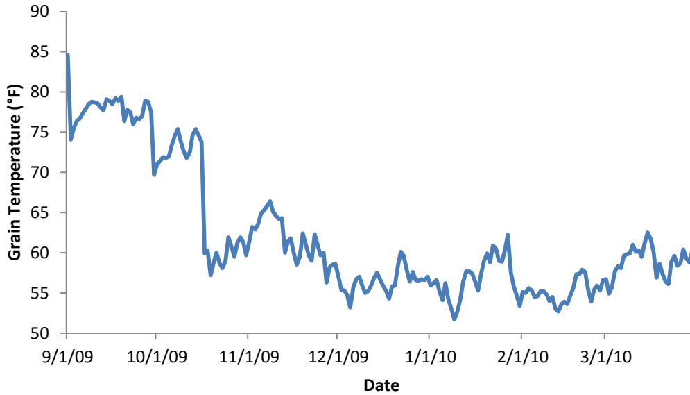
Figure III-13. Daily Grain Temperature for Rice Stored until March 31 st under Controlled Aeration Strategy.
