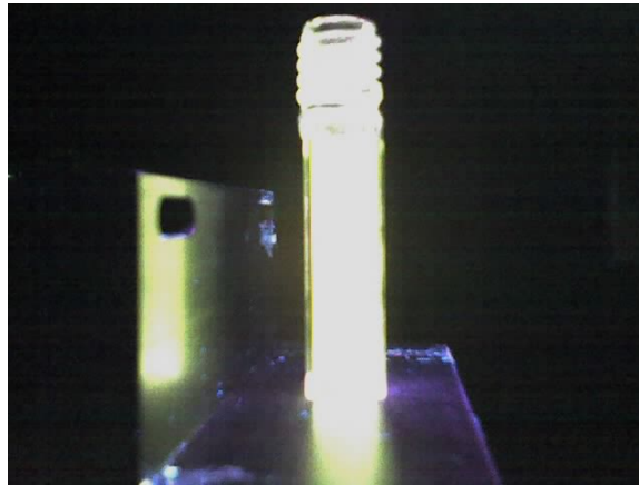
Figure 7.12: Photograph of a dilute CdS nanocrystal suspension excited with a mercury long-wave ultraviolet lamp. The particles are in water with 5% mercaptoacetic acid.
