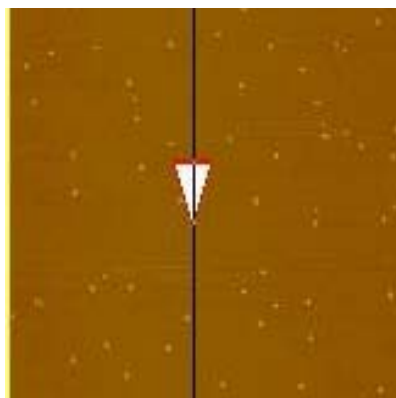
Figure 1. (a) AFM images of aggregates made by spin coating of the block copolymer (0.2 w/v) % in pS 48 -Cl ( 11 ) in THF; (b) Section analysis.
