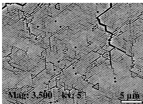
Figure 9. SEM image of the LCM packed by gravitational sedimentation and solvent evaporation with 10 wt % Texanol (sample 3, Table 1).
