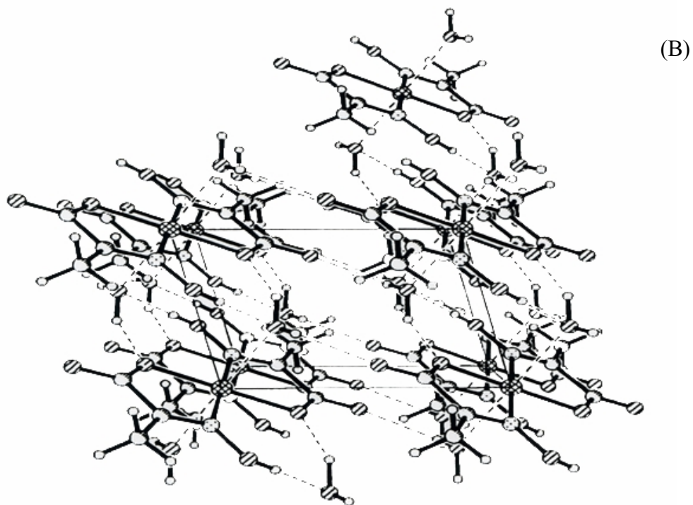
Figure 2.30. Perspective view of (A) the stacked chains of the copper complexes along the a-axis and (B) the extensive network of hydrogen bonds tying the copper complexes
